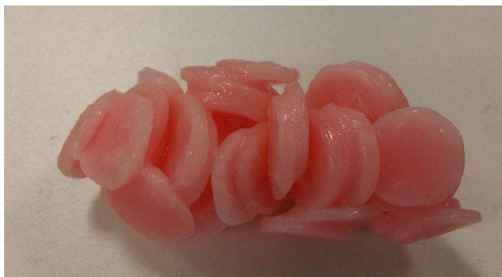
Figure 4.2: Example of damaged EverSoft® discs due to cleaning.
