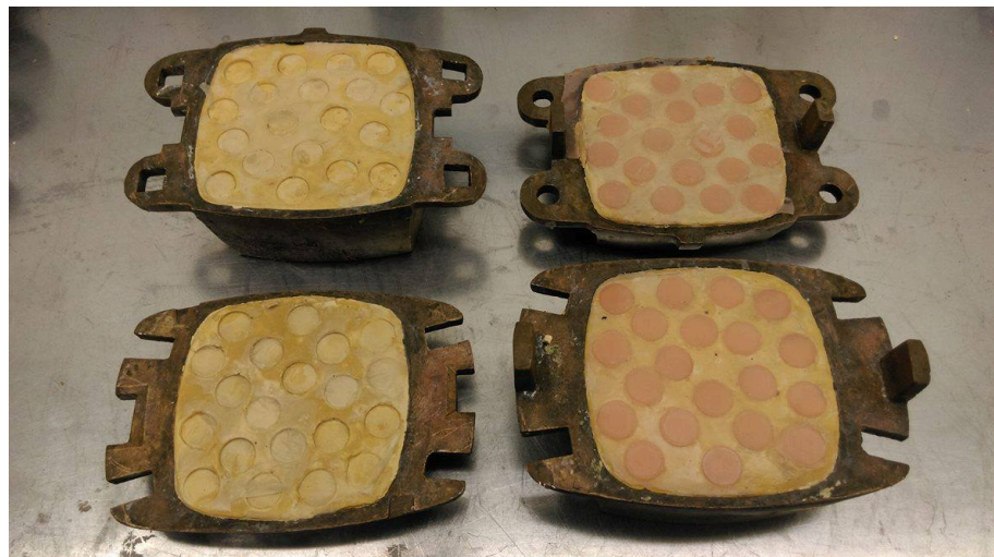
Figure 4.1: Example of the bespoke flasks used to fabricate discs of denture base materials.
