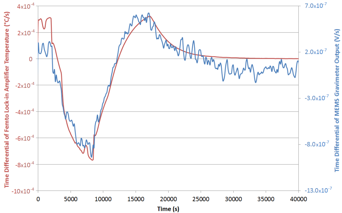
Fig. 5.4 A graph of the time differentials of the two series displayed in figure 5.3. The red series is the rate of change of the Femto temperature, \Delta T/\Delta t , and the blue series is the rate of change of the MEMS gravimeter voltage output, \Delta V/\Delta t . It can be observed that these two series are correlated – suggesting that output of the gravimeter is causally related to the temperature of the lock-in amplifier.
