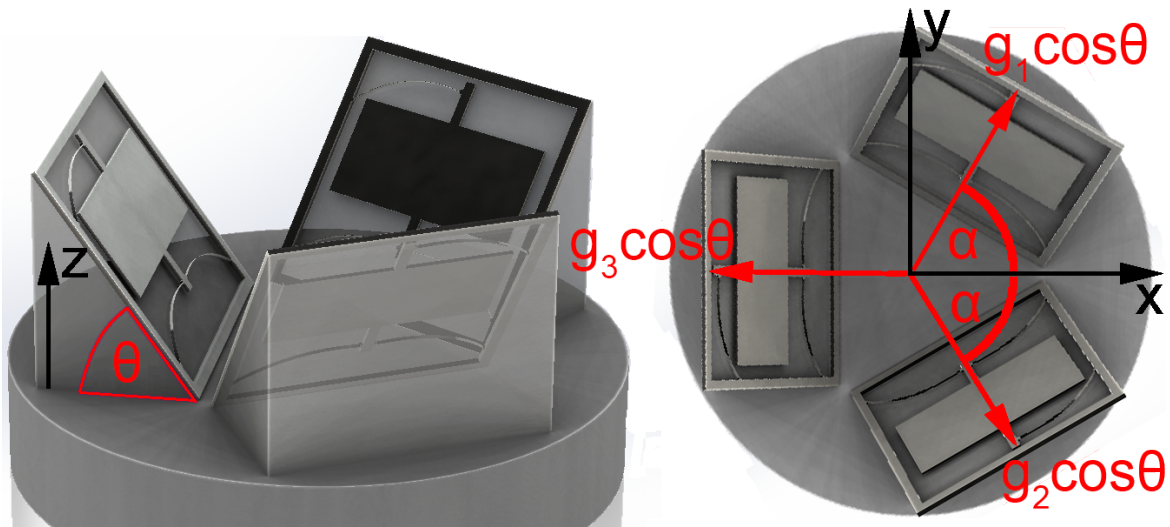
Fig. 2.12 A computer generated image of a three-axis MEMS gravimeter in a Galperin configuration [86].
