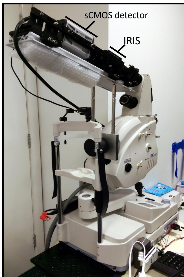
Figure 3-3. Topcon TR50-DX retinal fundus camera modified with IRIS and a sCMOS detector.
