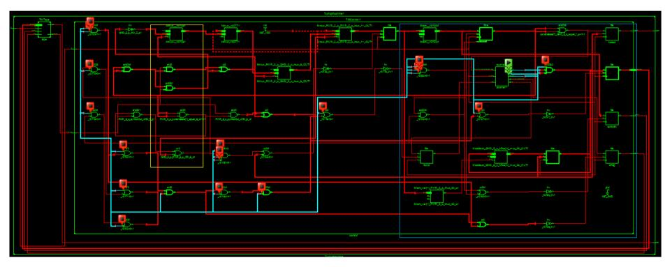
Figure 5.8: The RTL schematic of the TM control. The dark blue square contains the typically constant structures of the TM. The cyan connections are the output of the counter flip flop.
