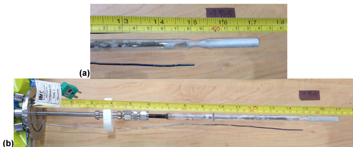
Figure 2-12: Polaris experiment: (a) sample placed at the bottom of the quartz tube for a total height of ca. 40 mm; (b) full experimental setup single glass quartz tube with inner stainless steel pipe for the flow of argon.
