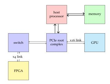
Figure 4.3: System architectural diagram showing interconnections between processors over PCIE network.
