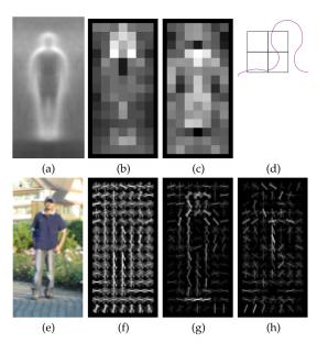
Figure 2.9: Building the нос processing pipeline. (a) Average gradient over training images. (b) Maximum positive svм weights in each block; (c) Maximum negative svм weights in each block; (d) Most relevant blocks (just outside contour); (e) Test image; (f) Hoc descriptor for test image; (g)–(h) Positive and negative weights for test image. Image and labels from [78].
