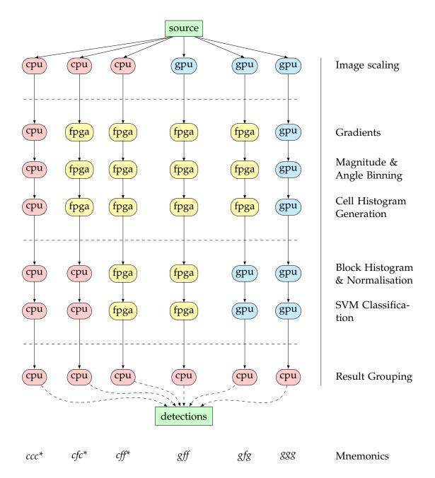
Figure 5.5: Six possible processing paths through the algorithm. Any one of these can be selected and used to generate detections. We define these using the three-letter mnemonics above in the format *resize-histogram-classify*. Starred mnemonics denote multithreaded versions.
