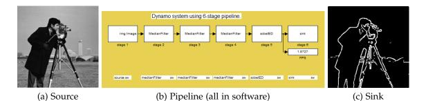
Figure 3.7: Sample image processing pipeline in Simulink, generated from implementations which were selected automatically. This performed repeated median filtering followed by Sobel edge detection, with each pipeline stage implemented in hardware or software.
