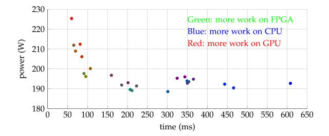
Figure 6.14: Power and time plots of all possible solutions, where each solution consists of one car HOG, one pedestrian HOG and the MOG detector, as described in Table 6.4. A greener dot represents a solution with most operations mapped to FPGA, while bluer and redder dots represent those with most operations mapped to CPU or GPU respectively.
