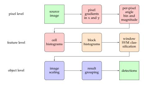
Figure 5.1: HoG algorithm stages: (i) gradients; (ii) angle & magnitude calculation; (iii) generation of oriented histograms over cells; (iv) block concatenation and normalisation; (v) linear svM scoring; (vi) image scaling; (vii) result grouping.
