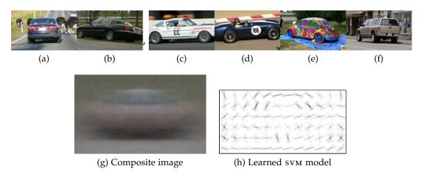
Figure 6.5: Example images for HOG car detector training. Composite of all training images shown in (g). Resulting detector model shown in (h).
