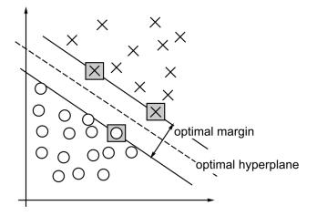
Figure 2.13: Support Vectors in a 2-D problem. The support vectors (grey squares) are placed on the optimal margin, which defines the largest separation between the two classes. Image from [89].
