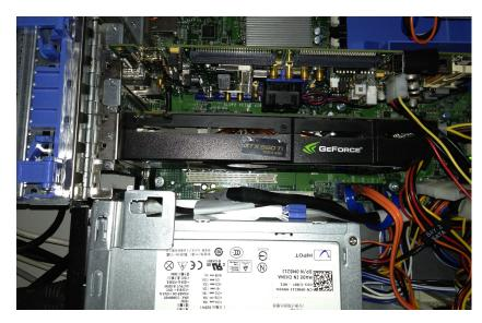
Figure 4.1: ML605 FPGA card (upper) and GPU card (lower) in development system.
