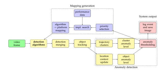
Figure 6.1: Frame processing and algorithm mapping loop in anomaly detection system. Figure 6.3 shows an expanded version of the "detection algorithms" block.
