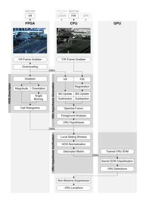
Figure 2.15: Processing pipeline in a hybrid system. Image from [70].
