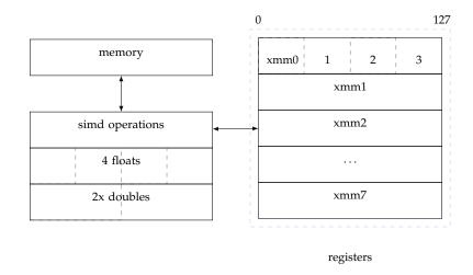
Figure 2.2: SIMD register structure in modern x86 processors. Eight 128-bit registers (right) can be used by the vector processing unit (left) for packed fixedand floating-point operations.
