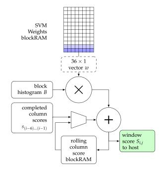
Figure 5.8: *C<sub>i</sub>*, one of eight block classifiers in a stripe. A block histogram is evaluated against each weight vector in turn and the result is accumulated into the classifier blockRAM. On readout, columns are summed together before adding completed column scores from the stripe to the left.
