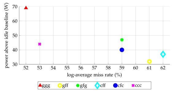
(a) Power vs. log-average miss rate plot using GTX560 GPU. Power consumption shown as increase over baseline of 147W.
