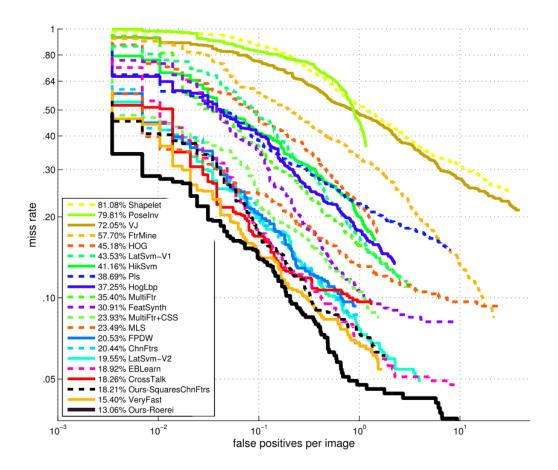
Figure 2.12: State-of-the-Art Pedestrian Detection Performance still requires improvement in many situations. INRIA dataset performance is shown in a Detection Error Tradeoff curve from [84].
