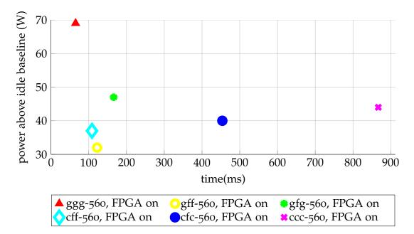
Figure 1.4: Run-time design space exploration: power vs. time for various implementations of HOG pedestrian detection using a GPU and FPGA. Power consumption shown as increase over baseline of 147W. Each version shown here can be selected at runtime. Letters denote the architecture which each algorithm segment is run on; *e.g.* for *gff*, resizing is done on GPU, followed by feature extraction and classification on FPGA.
