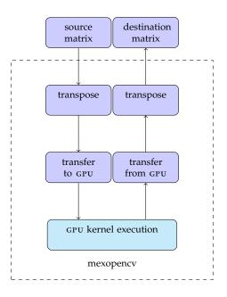
Figure 3.3: Running a GPU kernel in an OpenCV framework from within MATLAB.
