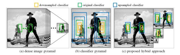
Figure 2.10: The Fastest Pedestrian Detector in the West moves away from the traditional approach of computing features and classifying on a densely sampled image pyramid (a). However, only scaling the classifier (b) does not work because the desired features are scale invariant. The hybrid approach (c) uses a classifier pyramid within each octave, but only samples and scales the image once per octave, considerably reducing evaluation time. Image from [81].
