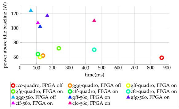
(a) Design-time design space exploration: power vs. time plot using small Quadro 2000 and large GTX560 GPU. Power consumption shown as use over baseline of 77W.
