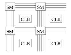
(a) Combinatorial logic blocks (containing look-up tables and storage elements) are connected by a configurable switch matrix.
