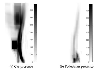
Figure 6.10: Presence intensity maps for different object classes in PV3. The colour bar denotes objects passing through that pixel, and the *x* and *y* axes correspond to the ground plane image of the scene (shown in Figure 6.8).
