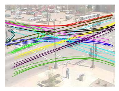
Figure 2.20: Offline filtered traffic analysis produces smooth detections. Image from [103].
