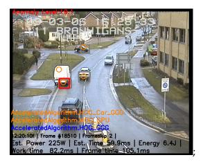
Figure 1.5: Real-time anomaly detection. The van parked on the left-hand side of the road is highlighted with a red square, signifying an anomaly. The overlaid text shows current system performance characteristics.
