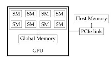
(a) Structure and memory interface of a streaming multiprocessor in a CUDA GPU.
