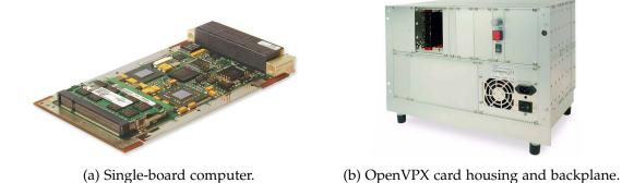
Figure 5.16: Single-board computer used in embedded system. OpenVPX backplane connection shown at top right.
