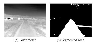
Figure 3.5: Road segmentation from IR polarimeter data.
