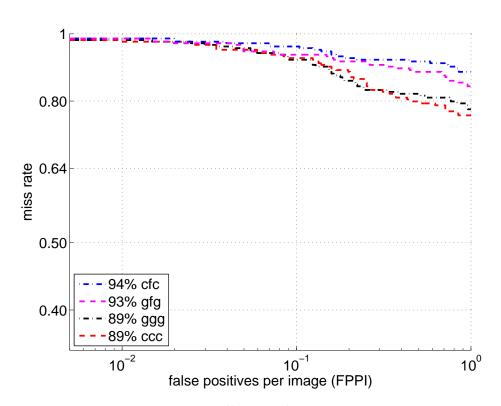
Figure 6.6: Detection Error Tradeoff curve for car detector implementations.
