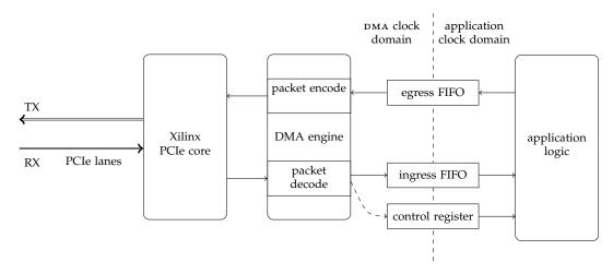
Figure 4.4: System internal FPGA architecture.
