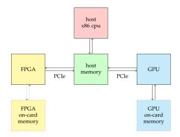
Figure 4.2: High-level system functional diagram showing arrangement of processors. Each processor can access host main memory, and the two accelerators have private access to on-card memory.
