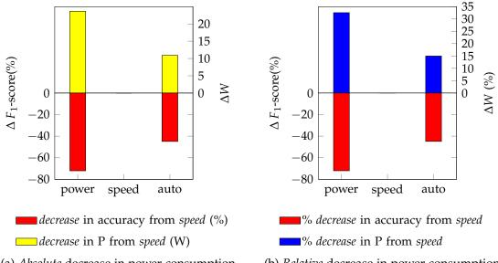
(a) Absolute decrease in power consumption and relative decrease in  $F_1$ -score of each configuration compared to *speed* prioritisation. (b) *Relative* decrease in power consumption and relative decrease in *F*<sub>1</sub>-score of each configuration compared to *speed* prioritisation.
