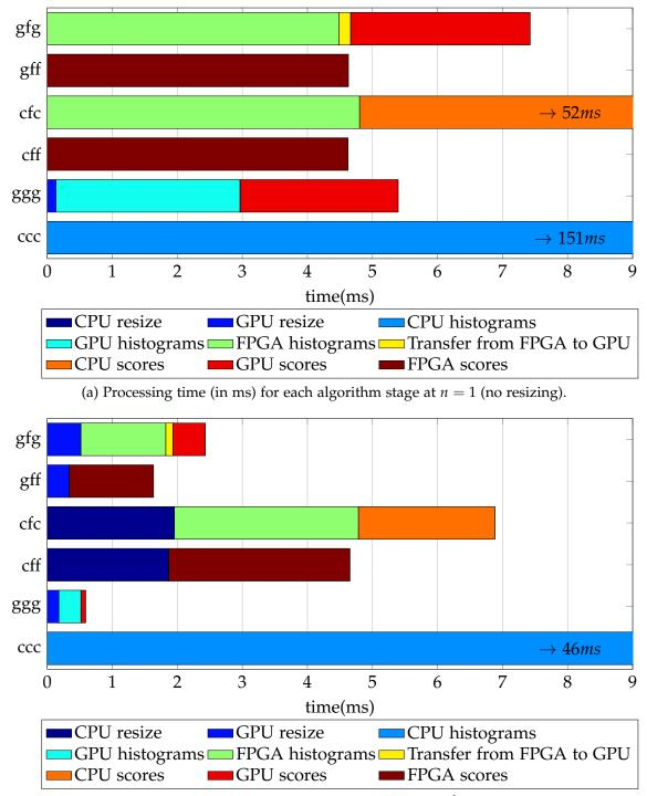
(b) Processing time (in ms) for each algorithm stage at  $37^{th}$  image scale only.
