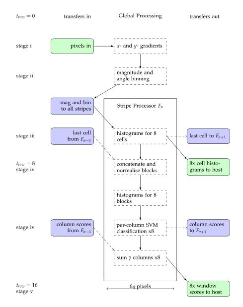
Figure 5.7: HoG stripe processors extract histograms from cells sequentially. Each stripe shares the normalisation logic, classification control logic and svm weights between its block classifiers. As pixels are fed in, cell histograms are generated, stored in an addressable shift register, and read out after 8 rows. Internally, these are then concatenated and normalised into block histograms. Cells from neighbouring stripes are included for blocks which overlap between stripes.
