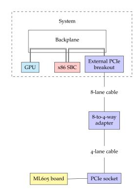
Figure 5.17: Embedded system connected to ML605 over PCIE. Packet loss suspected between system breakout and socket.
