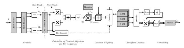
Figure 2.16: Fast FPGA HOG processing pipeline. Histogram generation steps shown. Image from [100].
