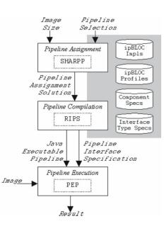
Figure 2.22: Pipeline assignment in the Dynamo system. Image from [60].
