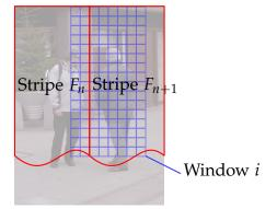
Figure 5.6: Processing regions for two stripe processors, overlaid on an image.  $F_n$  passes cell histograms and column scores for the left portion of window *i* to  $F_{n+1}$ .
