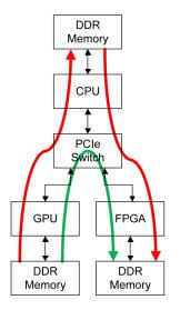
Figure 2.6: Reduced transfer times between FPGA and GPU are achievable by initiating a DMA transfer directly between the two device memories (green) rather than an intermediate copy to host memory (red). Image from [14].
