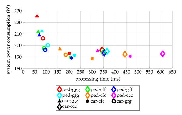
Figure 6.15: Power and time plots of all possible solutions, where each solution consists of one implementation of car HOG, one for pedestrian HOG and the MOG detector, as described in Table 6.4. Pedestrian implementations are labelled by colour, and car implementations by shape; thus the dark blue hollow circle at t = 95ms means a solution with pedestrian HOG mapped to *gff*, car HOG mapped to *gfg* and MOG, as always, mapped to *GPU*.
