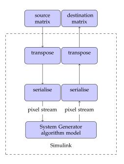
Figure 3.2: Modelling a FPGA algorithm using System Generator for Simulink from within MATLAB.
