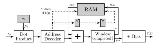
Figure 2.17: Fast FPGA HOG processing pipeline. Classification steps shown. Image from [100].
