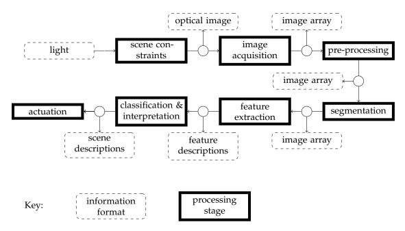
Figure 2.1: Image Processing Pipeline (from Awcock & Thomas [18]). Each stage in the pipeline can be considered another layer of abstraction.
