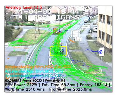
Figure 6.9: Learned object clusters, projected onto camera plane. Green, blue and orange tracks represent cars, pedestrians and undetermined (motion-only) objects respectively.
