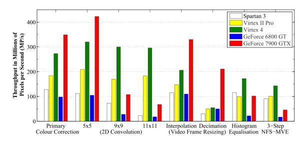
Figure 2.5: Throughput of image processing operations on 3 FPGAs and 2 GPUs compared. Image from [67].
