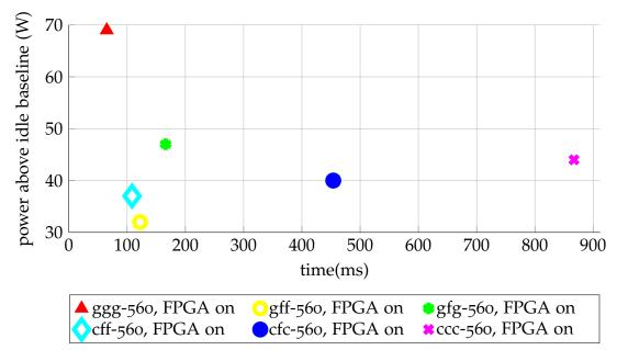
(b) Run-time design space exploration: power vs. time plot using GTX560 GPU. Power consumption shown as increase over baseline of 147W.
