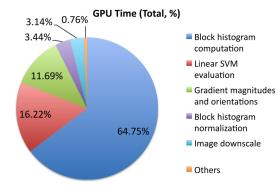
Figure 2.14: Time spent on each algorithm stage in a HOG GPU implementation. Image from [96].
