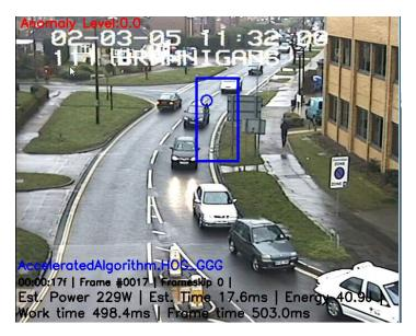
Figure 6.4: False positive (blue rectangle) from нос pedestrian detector. Similar problems affected the car detector.
