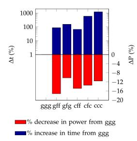
(a) Relative change in processing time and power consumption of each configuration compared to *ggg*. A red bar below zero indicates decreased power consumption.
