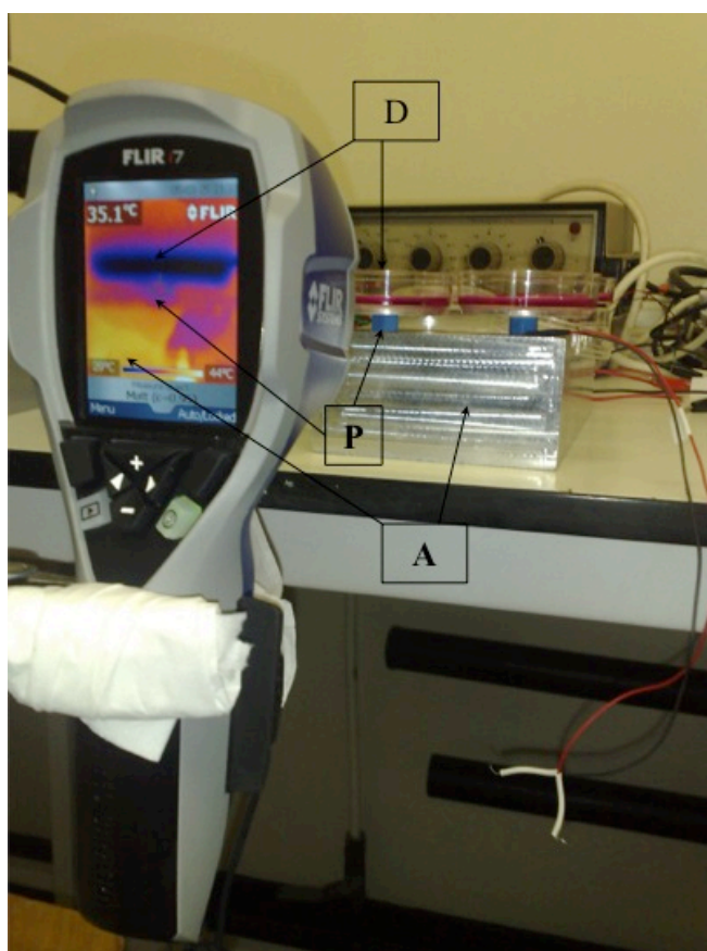
Figure 3-9- Thermal imaging setup: Thermal camera is placed in position providing a side-view of two Petri dishes, mounted on top of the piezo actuators and aluminium block respectively. The infrared emission can be observed on the camera display, showing the cold media (D) due to evaporation, a warmer pink point underneath the piezo actuator (P) and yellow background from the aluminium block (A).
