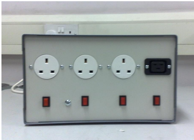
Figure D-1: Purpose-built power analyser unit with three standard 13A sockets and a 10A phase-controlled output.
