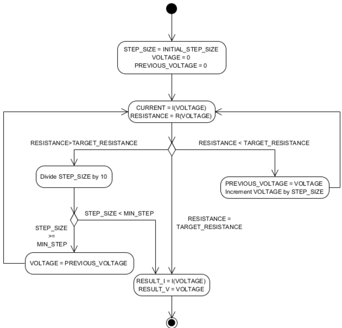
Figure 4-5: Illustration of the new algorithm developed to determine the operating point of a solar panel when the load resistance is known. The output current I(V) is obtained using (23) and R(V) = V/I(V) .
