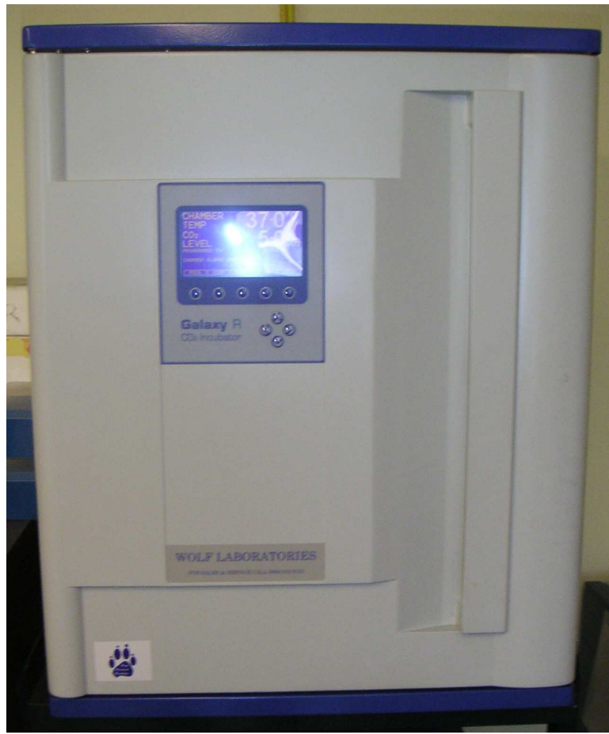
Figure 2.8 Galaxy-R Hypoxic Chamber: Humidity, O 2 and CO 2 Regulated
