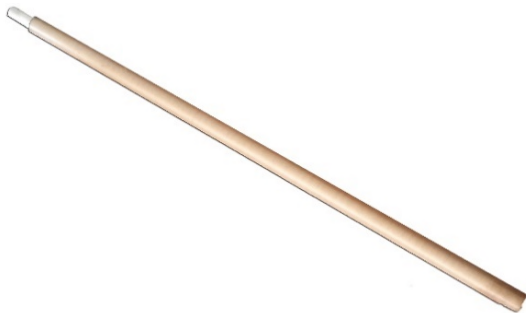
Figure 4: Mandrel used for fabrication of shafts
