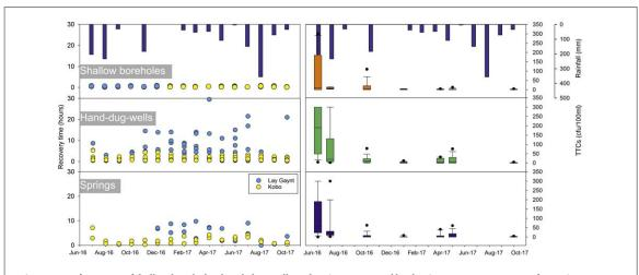
**Figure 3.** Performance of shallow boreholes, hand-dug-wells and springs measured by the time to recover to 50% of morning rest water level, monthly rainfall over the period from TAMSAT is shown for comparison. Summary TTC measurements at different times of the year for all measured sources are shown on the right: 15 shallow boreholes 17 hand-dug-wells, and 19 springs table S2 gives summary statistical data.
