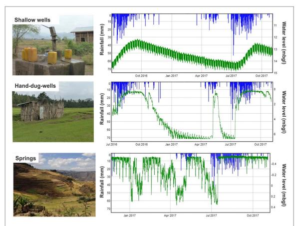
Figure 2. Examples of measured groundwater level in three monitored sources (green): shallow borehole, hand-dug-well and springs with weekly rainfall totals from TAMSAT for comparison (blue). For the spring, the water-level is the level in the spring box reservoir. Rainfall Data TAMSAT $^{\odot}$  University of Reading (Maidment et al 2017).
