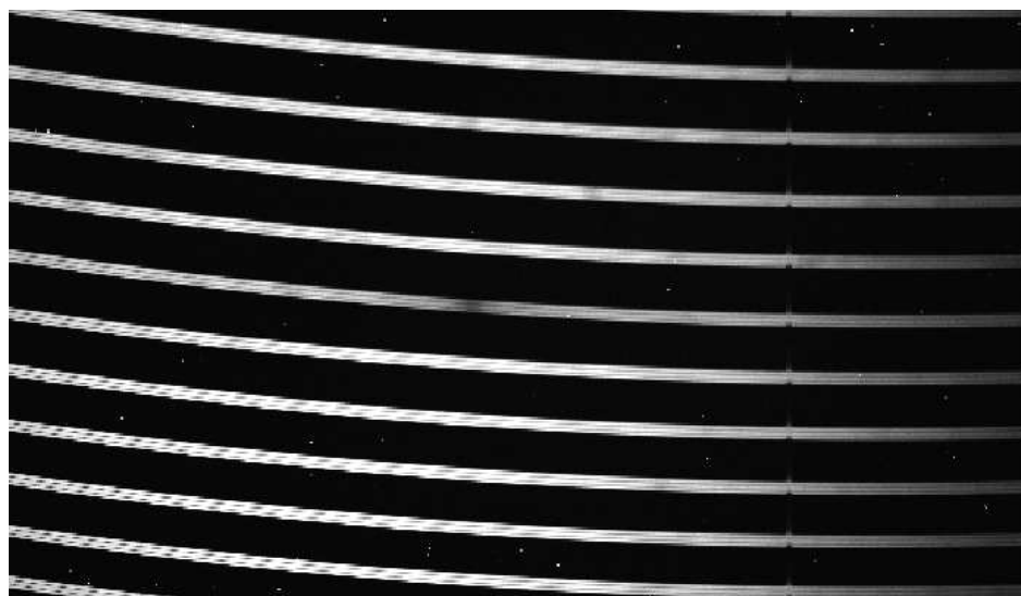
Figure 5.4: A section of the image of a dispersed spectrum from an echelle spectrograph (SALT/HRS). The many spectral orders have been separated with a 2 nd order cross-disperser. The spectral dispersion direction is the x-axis, and the order dispersion is in the y-axis. The spectrum has not been corrected for instrumental sensitivity.
