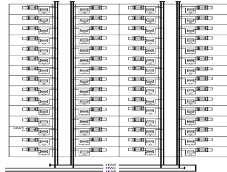
Figure 4. Layout of piping in building
