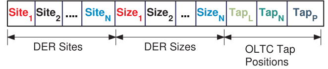
Fig. 2. The structure of individual used in the proposed MSO for DER integration in conjunction to OLTC tap control.
