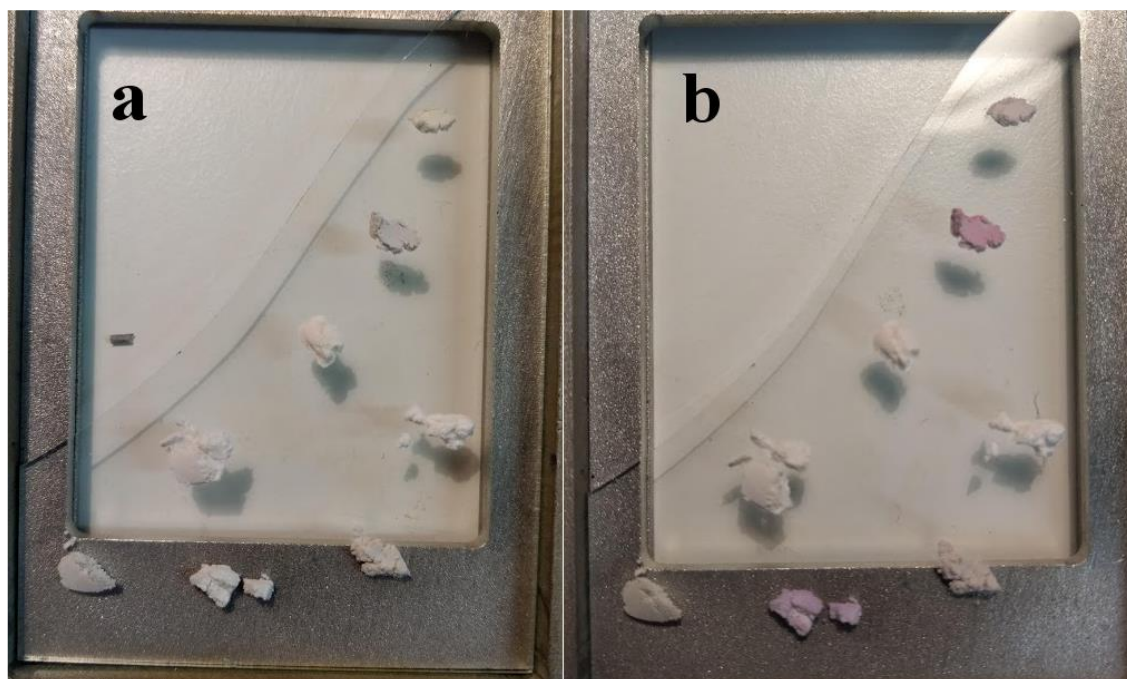
Figure 7. Various hackmanite samples a) before exposure b) after exposure to an electron beam in a cathodoluminescence setup.
