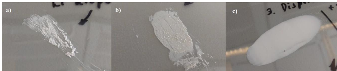
Figure 17. The treatment results. All the tapes are cast onto a PET film with a another piece of the same film a) No dispersant; mixing in a test tube with a laboratory spatula b) Mixing the ceramic powder, the solvent and the dispersant in a planetary grinding mill (Philips Minimill PW4018/00) for 10 minutes at speed 1; mixing BBP and PVB with a spatula c) The ceramic powder ground with a planetary grinding mill for 10 minutes at speed 1; mixing the powder with the solvent and the dispersant for 10 minutes at speed 1 in a planetary grinding mill; mixing BBP and PVB with the suspension for 2 minutes at speed 1 in a planetary grinding mill.
