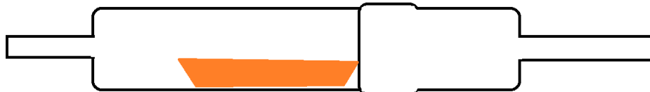
Figure 14. Alumina crucible (orange) in a quartz reactor (inlet and outlet not sealed).
