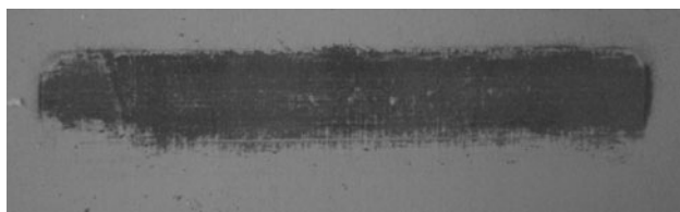
Fig. 19 Oxide coating representing the counter-specimens after the tribological tests [19]
