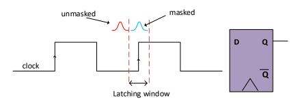
Figure 2.18: Illustration of latching-window masking where the transient pulse reaches outside the latching window of a flipflop.
