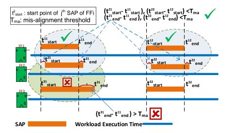
Figure 4.3: Correlation analysis of flip-flops based on the overlap of concurrent SAPs.
