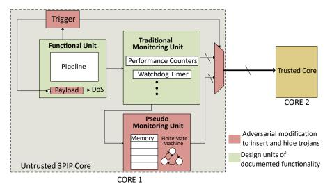
Figure 6.2: Illustration of a Trojan attack scenario including manipulation of architectural-level monitors to mask the attack.
