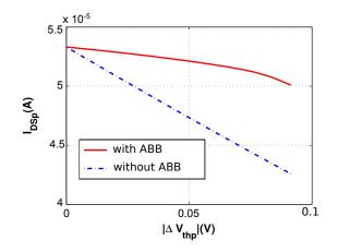
Figure 2.13: Illustration of the driving strength  $((I_{DSp}))$  of two aging-stressed PMOS transistors, one with and the other without adaptive body biasing [20].
