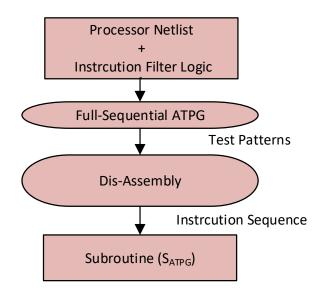
Figure 4.4: Flow chart showing the steps involved in ATPG-based subroutine generation
