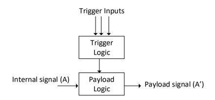
Figure 2.19: Illustration of a hardware Trojan architecture with a trigger logic and payload.
