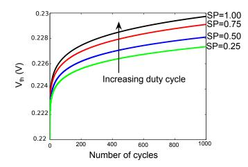
Figure 2.8: The dependence of  $V_{th}$  on signal probability (SP) [44]
