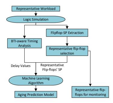
Figure 3.2: Flow-chart showing the steps involved in the offline characterization phase.
