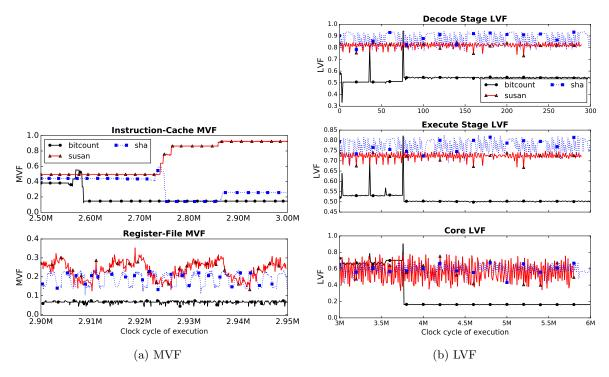
Figure 5.1: The VF of the memory arrays and sequential logic blocks in Leon3 for three MiBench workloads (experimental setup described in Section 5.7).
