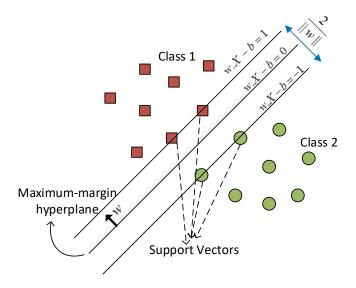
Figure 2.21: Illustration of linear two-class classification with maximum-margin hyperplane in support vector machines.
