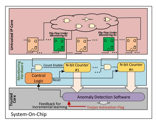
Figure 6.6: Illustration of runtime monitoring hardware and anomaly detection
