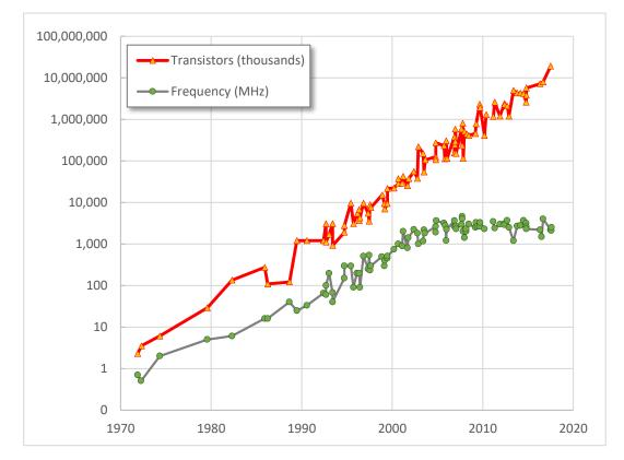
Figure 1.1: Illustration of complexity and performance increase with technology scaling advancement in microprocessors for the last four decades [1].
