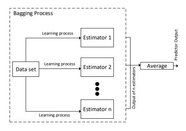
Figure 2.24: Illustration of bagging technique.
