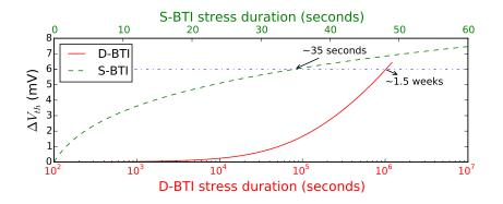
Figure 2.5: Comparison of  $\Delta V_{th}$  due to D-BTI (duty cycle ( $\alpha$ )=0.5) and S-BTI.
