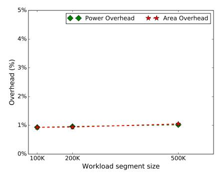
Figure 5.12: Variation of overheads with workload-segment size for Leon3 processor.
