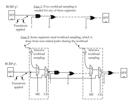
Figure 2.12: Representative critical reliability paths showing representation of critical paths with or without workload sampling [47].
