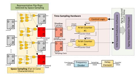
Figure 3.6: Illustration of flip-flop SP monitoring methodology.
