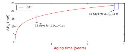
Figure 3.1: The difference in  $\Delta D_{min}$  at different time points in the lifetime of a circuit.
