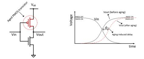
Figure 2.6: Illustration of an aged CMOS inverter (INV1) and the corresponding deviation in inputouput characteristics in the form of an additional delay in the switching functionality.
