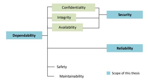
Figure 2.1: Illustration of the attributes of dependability in the scope of this thesis [8].
