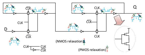
Figure 4.9: Illustration of static aging relaxation of the internal transistors of a master-slave flip-flop on subsequent switching events.
