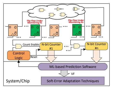
Figure 5.7: Illustration of flip-flop SP monitoring methodology.
