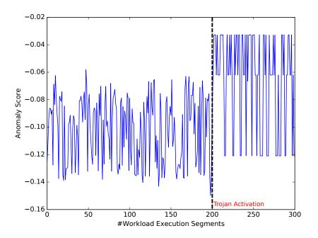
Figure 6.7: Illustration of the shift in anomaly score when the NOP-insertion Trojan is activated during the execution of a susan\_smooth application in Leon3.
