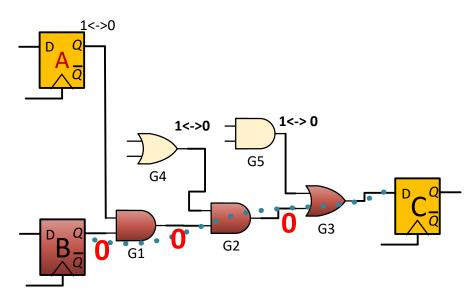
Figure 4.8: Illustration of switching event propagation from flip-flops under static aging to the logic gates under static aging in their forward fanout cone.
