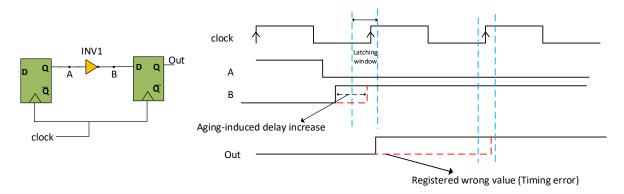
Figure 2.7: Illustration of a timing violation and failure caused by an aging-induced delay increase in a timing path.
