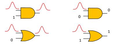
Figure 2.16: Illustration of logical masking or propagation of transient pulse from the input of a logic gate for different input combinations.
