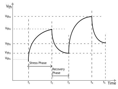
Figure 2.4: Illustration of stress and recovery phases due to NBTI
