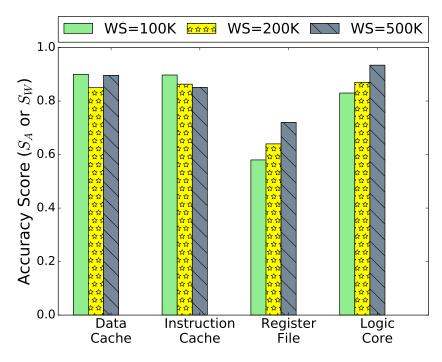
Figure 5.11: Variation of prediction accuracy with workload-segment size (WS) for different hardware structures in Leon3.
