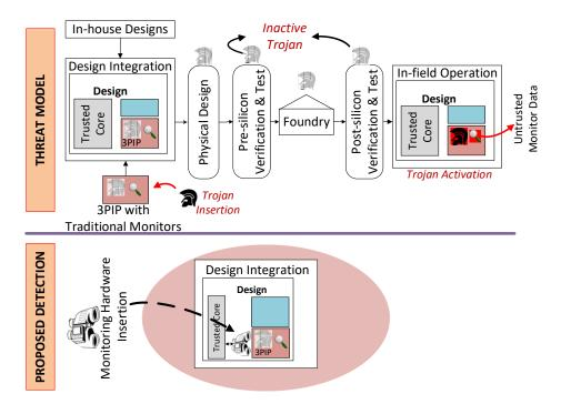
Figure 6.1: Threat model showing stages of Trojan insertion and activation in SoC design flow along with the proposed detection technique.
