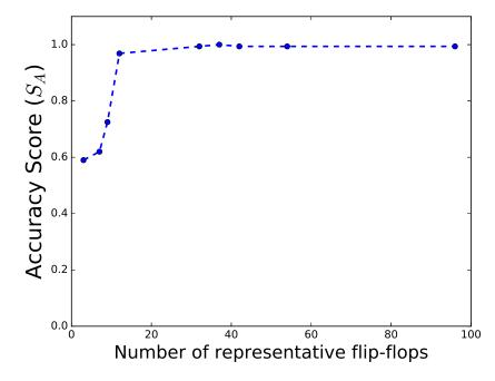
Figure 6.10: The variation in prediction accuracy of Trojan activation in Leon3 with the number of flip-flops selected for monitoring.
