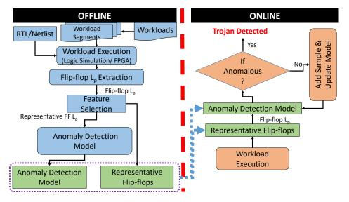
Figure 6.3: Proposed flow showing offline characterization, prediction model construction and its online deployment.
