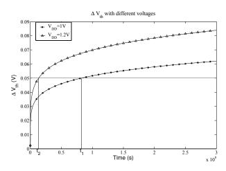
Figure 2.14: Illustration of the dependence of NBTI-induced threshold voltage degradation on supply voltage [19]
