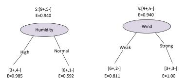
Figure 2.23: Illustration of information gain comparison between two attributes [66].
