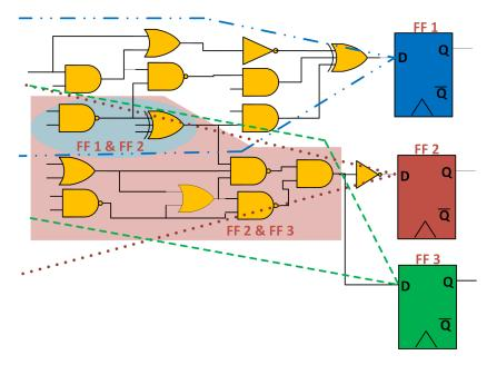
Figure 3.5: Fan-in cone characteristics of flip-flops.
