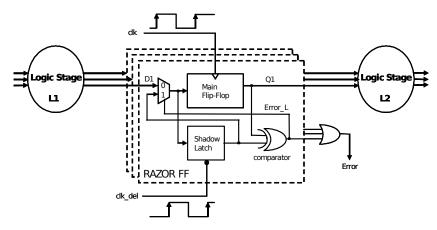
Figure 2.9: Razor flipflop deployed in a timing path to monitor the delay and restore the correct value in case of a timing error [22].
