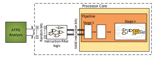
Figure 4.5: Illustration of ATPG-based subroutine generation settings for mitigating static aging.
