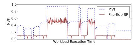
Figure 5.2: Variation of instruction-cache MVF of Leon3 and SP of a selected flip-flop during MiBench workload execution.
