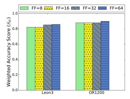
Figure 5.10: Variation in Weighted Accuracy Score  $(S_W)$  for LVF prediction with the number of representative flip-flops selected for Leon3 and OR1200 logic cores.
