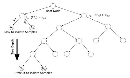
Figure 6.5: Illustration of a random decision tree for isolating samples.
