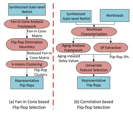
Figure 3.4: Overall flow of space-sampling techniques to identify representative flip-flops.
