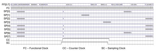
Figure 3.8: Timing simulation results for the time-sampling hardware.
