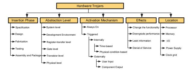
Figure 2.20: Hardware Trojan Taxonomy based on different characteristics of Trojans [61]
