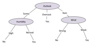
Figure 2.22: Illustration of a decision tree demonstrating a two-class classification [66].
