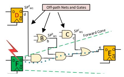
Figure 5.5: Flip-flop SEU due to particle strike and error propagation scenario in a timing path.
