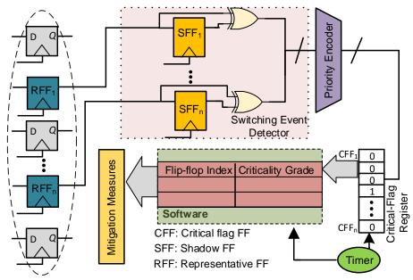
Figure 4.7: Illustration of the online static aging monitoring hardware.
