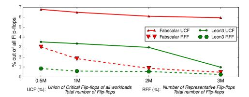
Figure 4.10: Results demonstrating the variation in percentage of (a) union of critical flip-flops of all workloads (UCF), and (b) representative flip-flops (RFF), with the minimum duration of SAPs for Fabscalar and Leon3 processors.
