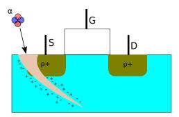
Figure 2.15: Effect of alpha-particle strike on a transistor eventually leading to soft error.
