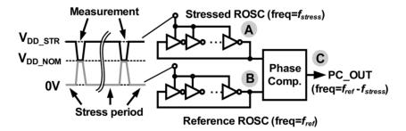
Figure 2.10: Illustration of BTI monitoring by measuring the beat frequency between two ring oscillators with one of them under stress and the other used as a reference [45].
