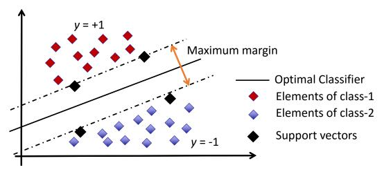
Figure 5.6: Illustration of two-class SVM classification.
