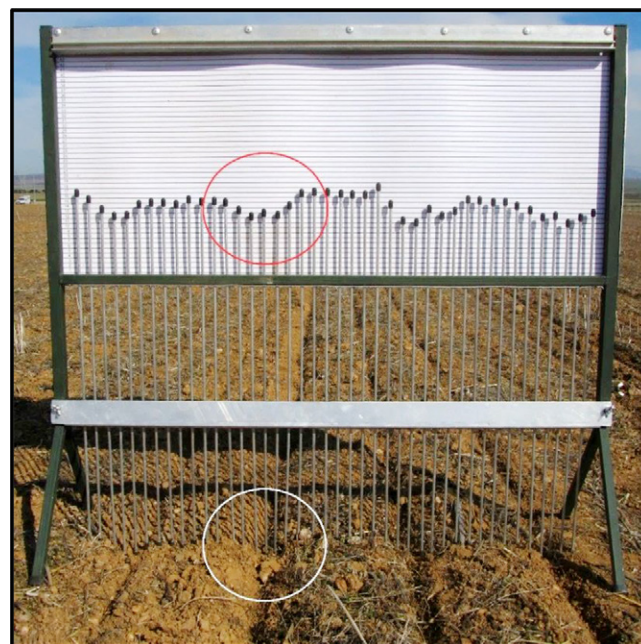
Fig. 2. Pin profiler used to determine the amount of aboveground soil disturbance. The white circle at the bottom indicate the furrow in the soil caused by the opener, while the red circle at the top indicates the roughness profile of the furrow.
