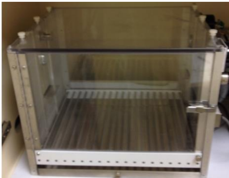
Figure 2.2. Contextual fear conditioning chamber. Identical chambers within a common testing room served as the fear conditioning and memory retention testing contexts. Each rat was conditioned and tested in the same chamber.
