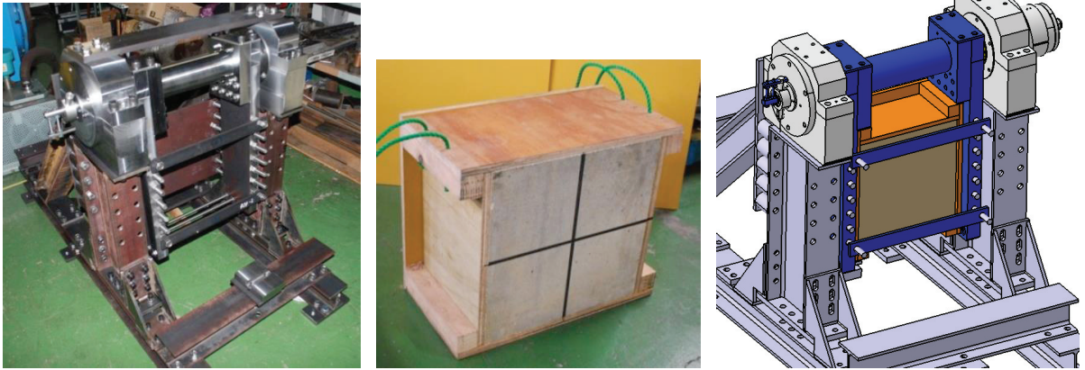
Fig.3. Images of our pendulum: left shows appearance of pendulum (about 400 kg); center shows bricks target (300×300×t140, 28.65 kg, 2.27 g/cm 3 ) with wooden frame (plaster as other targets); right shows pendulum with target.
