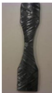
Figure 4: Specimen for a tension test which was cut down from the CFRP circular
