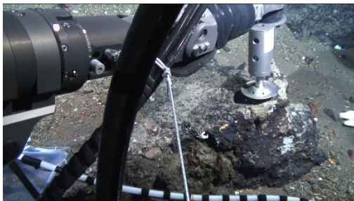
3Grinding machine operating on rocks in the ocean
