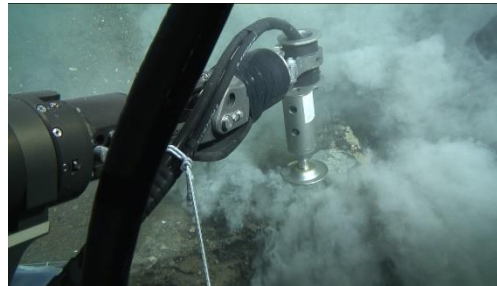
3Grinding machine operating on rocks in the ocean
