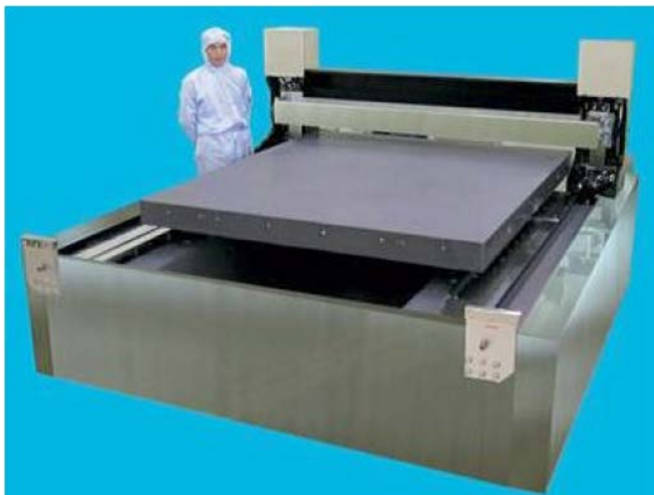
Fig. 1.3 Resin coating machine for liquid crystal panel [20]
