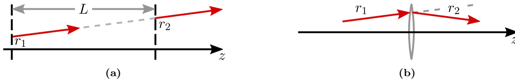
Figure 4.11: (a) Schematic of free ray propagation over a distance L , changing the transverse distance r to the optical axis z . (b) Schematic of refraction of a ray at a lens, changing the slope dr/dz (adapted from [105] ).
