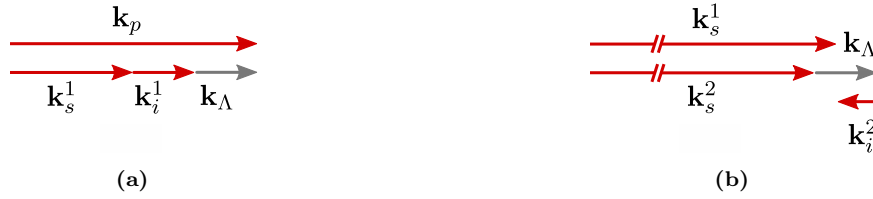
Figure 4.15: (a) Schema of the quasi wave vector mismatch for the ideal OPO operation. (b) Conversion to an additional wave with k_s^{(2)} caused by backward oscillation of an idler wave with k_i^{(2)} (adapted from [116] ).
