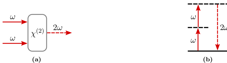
Figure 4.1: (a) Schema of geometric beam propagation after SHG. (b) Schema of the SHG energy level diagram. The virtual levels are represented by dashed lines (adapted from [91] ).
