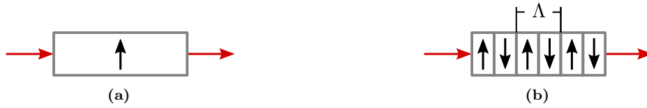
Figure 4.6: (a) Schematic of a homogeneous medium with one optical axis \hat{c} . (b) Schematic of a periodically poled medium with an alternating optical axis and the period length \Lambda (adapted from [91] ).
