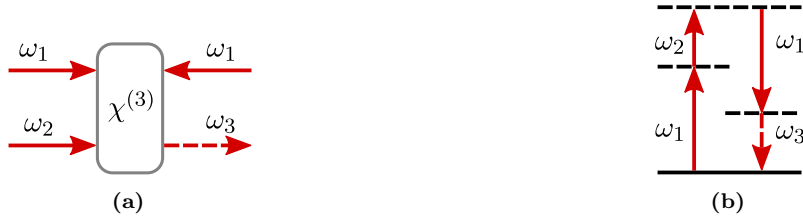
Figure 4.4: (a) Schematic of the four wave mixing process in the MTS setup. Three collinear photons get destroyed in favor of a fourth photon at \omega_3 = \omega_2 . (b) Energy level diagram of the four wave mixing process, with dashed virtual levels (adapted from [91]).
