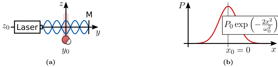
Figure 8.7: (a) Schema of a single molecule passing perpendicular a standing wave, with a well defined position of the molecule along the y -axis. (b) Schema of the Gaussian power distribution of the electric field along the x -axis.
