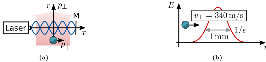
Figure 8.3: (a) Schematic of a laser retroreflected at a mirror M, with an atom beam moving perpendicular through the light field. The individual atom is delocalized inside the standing wave. (b) The field distribution of the standing wave has a Gaussian line shape along the propagation direction of the atoms.
