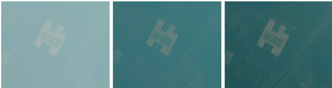
Figure 4.2: A closer look at the images from Figure 4.1 demonstrating the original hazy image, atmospheric scattering, and Perlin noise data generation methods
