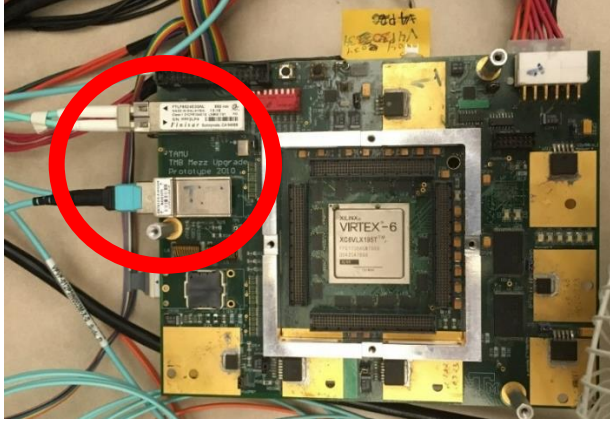
Figure 2: Test Board for last series of radiation tests w/ tested components
