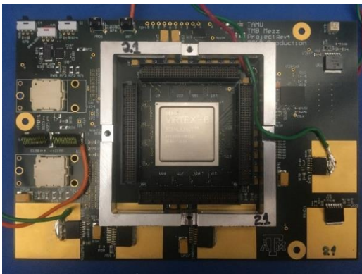
Figure 4. March 2017 Test Board for LDO devices. The devices sit on copper cooling pad.
