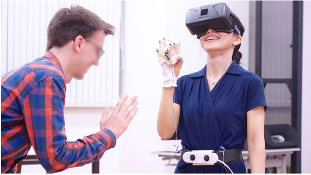
Figure 3: A wearable visual device that allows a user to change their body representation, in realtime, to that of a small-person
