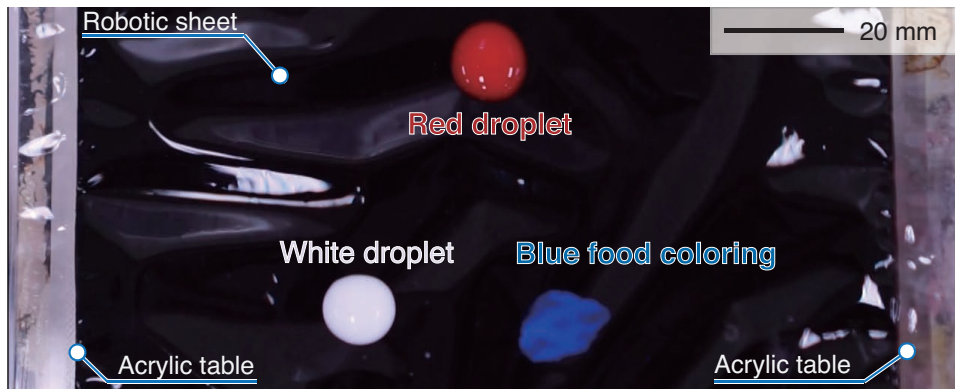
FIGURE 5.11: Initial state of the liquid application experiment. Transportation and mixing are conducted in one sequence. At first, a white droplet moves to a red droplet. After these droplet are combined, the combined droplet are mixed using oscillation. The mixed droplet moves to blue powder, and the droplet and powder is mixed.
