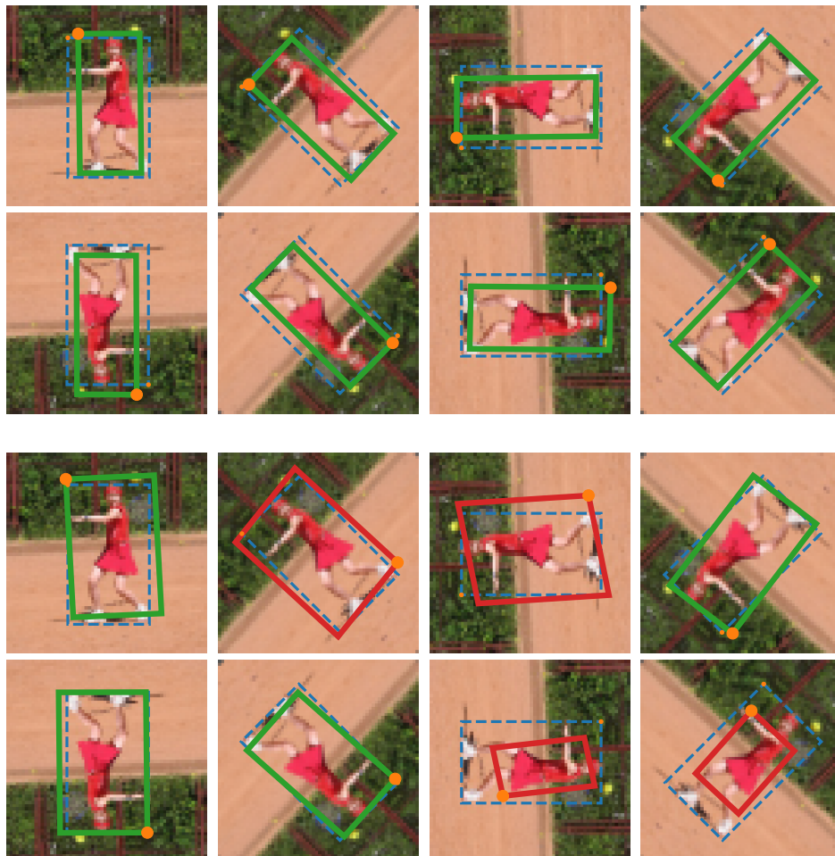
Figure 4.8: Estimation results of the bounding box regression (1/3). Upper images are the results of the proposed method, Architecture (d). Lower images are results of Architecture (a). Green box denotes true positive. Red box denotes false positive. Blue dash box denotes ground-truth box. Orange dot denotes the upper left corner of the bounding box. Threshold of OIoU is 0.5. The original images are from the website: https://www.flickr.com/photos/impuls-f/2434568700 .
