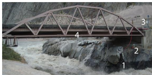
Figure 2: The monitoring station at Watson River: 1. sensors (Solitech 10, OBS3+); 2. automatic pump sampler (ISCO); 3. datalogger box; 4. radar water level (Ott).
