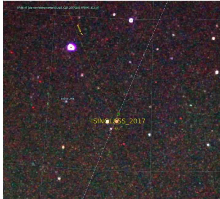
Figure 12: Identification and Subsequent ray tracing analysis outputs position information in the form of geodetic longitude, latitude, and altitude. The yellow ray (top left to bottom right) represents trajectory of the highlighted Bob from Venetie, and the white ray (bottom left to top right) is the trajectory of the main payload.
