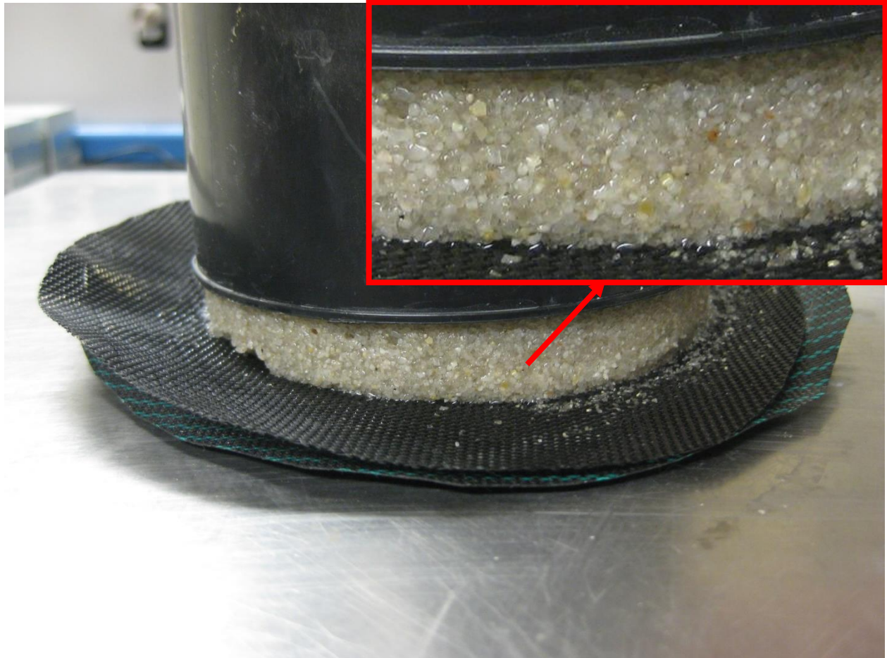
Figure 2.5 Capillary water in sandy soil
