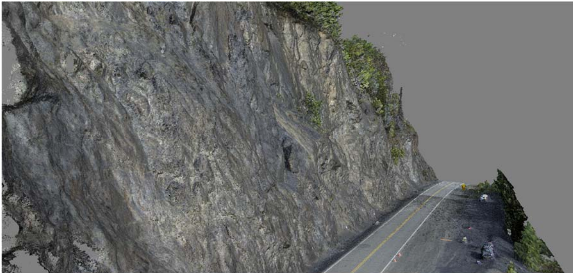
Figure 8 - DSM model example from UAS imagery and SfM processing
