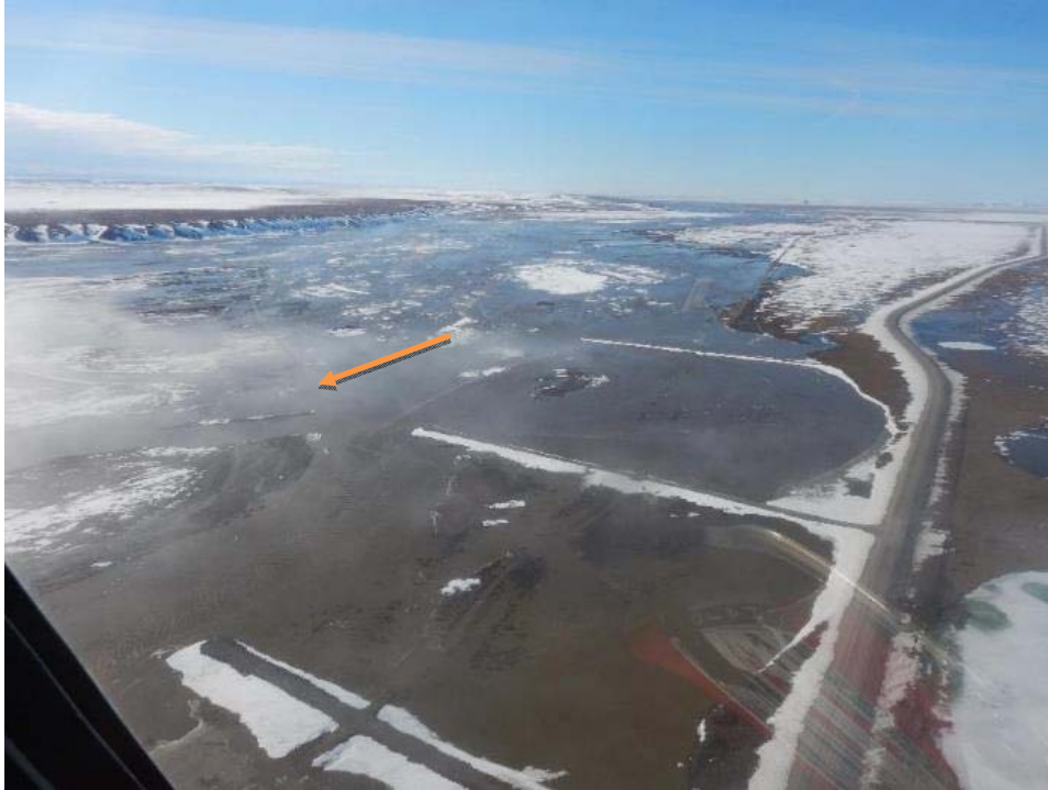
Figure 65. A south-facing view of the Sagavanirktok River on May 28, 2017. On the right is the Dalton Highway—perpendicular structures are spur dikes over the buried pipeline. Franklin Bluffs is visible in the distance to the left.
