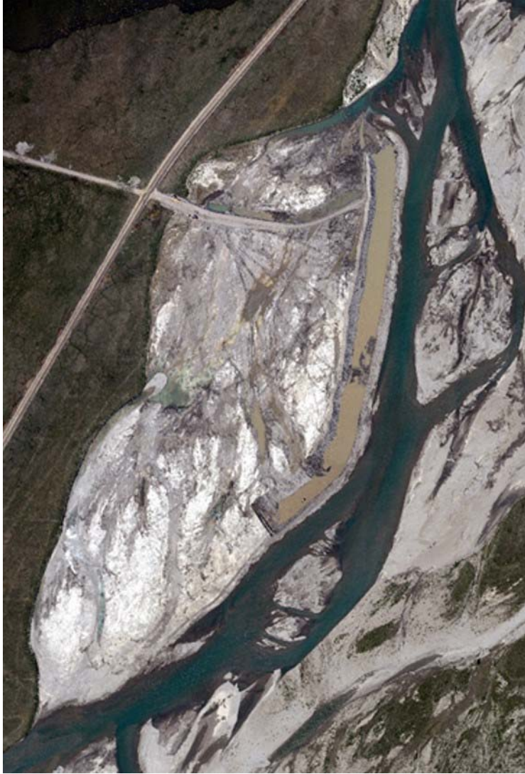
Figure 9. Aerial photograph showing gravel mining on the west channel of the Sagavanirktok River near Dalton Highway MP405 (station DSS1 is approximately 1.5 km downstream).
