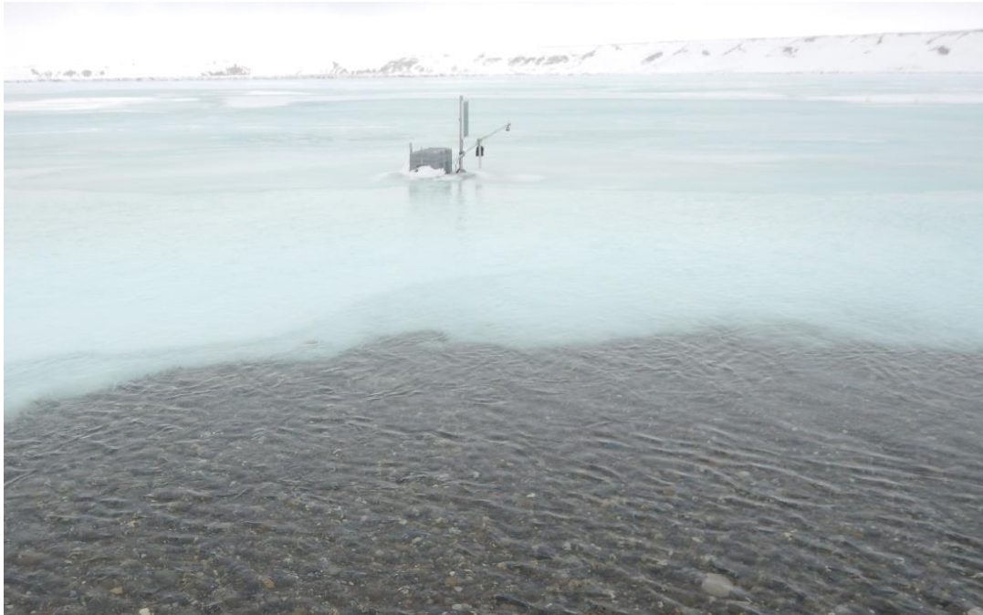
Figure 39. SR50 sensor at MP387.5 on May 3, 2016, recording overflow and growth of aufeis.
