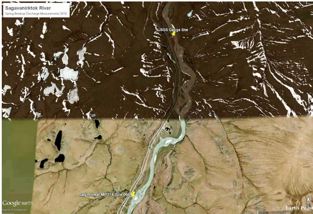
Figure 7. Locations of 2016 flow measurements on the Sagavanirktok River near MP318 (DSS4). Most of the measurements were made at the USGS gauge site during breakup.
