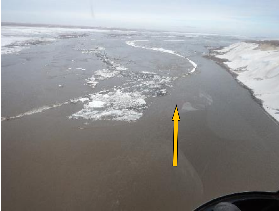
Figure 61. Slightly higher water levels on the Sagavanirktok River at Franklin Bluffs overtop the ice berm above its constriction on May 20, 2016. Gravel and aufeis are once more submerged. View is north.
