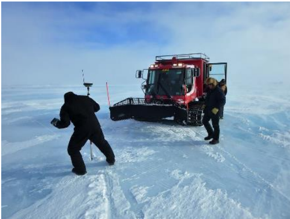
Figure 29. UAF researchers and ADOT&PF surveyors map elevation and thickness of aufeis formations on Sagavanirktok River near Franklin Bluffs on April 19, 2016.
