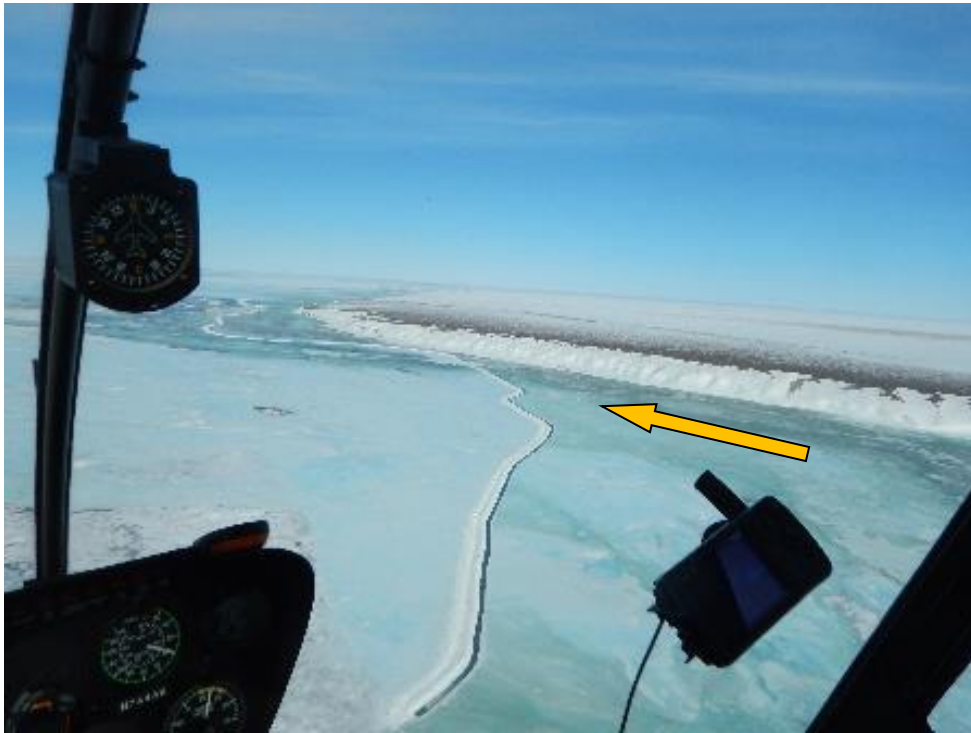
Figure 55. This northward view shows aufeis on Sagavanirktok River at Franklin Bluffs and easternmost trench and berm in its initial condition on May 10, 2016. Note acute narrowing of trench and berm with the Bluffs at mid-photo.
