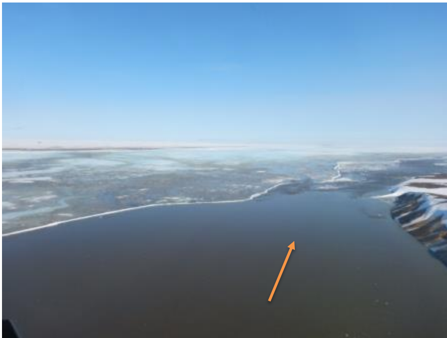
Figure B.22. Photo taken May 16, 2015, near bifurcation of the Sagavanirktok River. View is north. Photo shows a large amount of water being directed to the East Fork by a diversionary snow dike with extensive aufeis beyond. Dark linear streak near horizon is Dalton Highway. Franklin Bluffs are east (far right).
