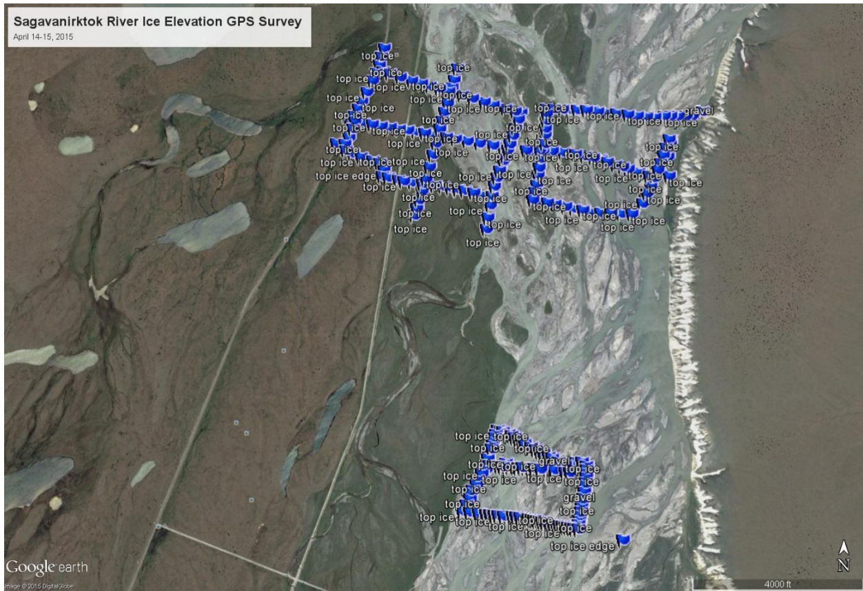
Figure 12. Locations of points surveyed with a GPS to map ice elevation near Franklin Bluffs.
