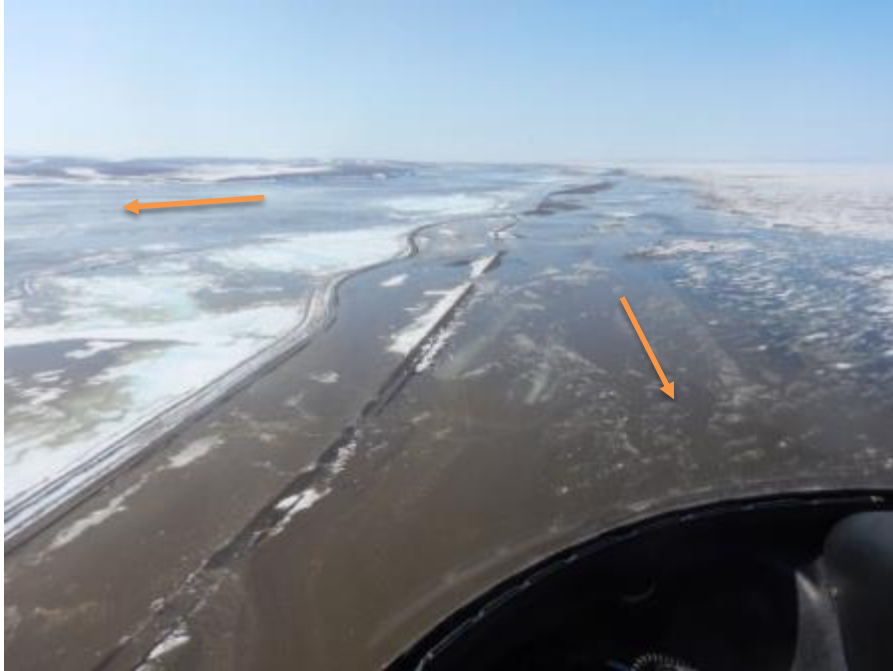
Figure B.5. Photo taken May 18, 2015, near Dalton Highway MP400, view south. Photo shows water levels rising and inundation of tundra west (right) of the pipeline. A Sagavanirktok River channel is at far left, and Franklin Bluffs are seen in the distance, upper left of center.
