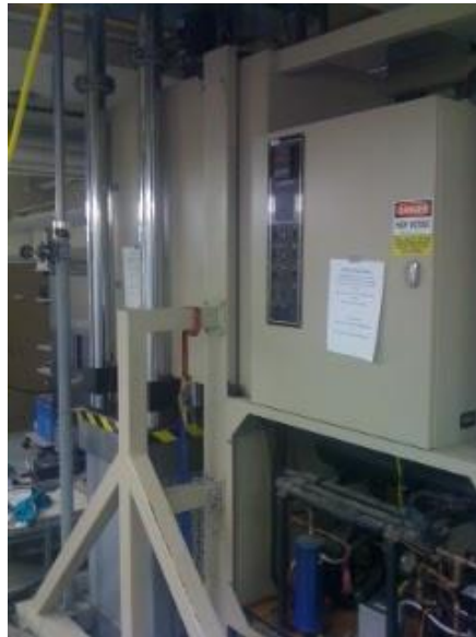
Figure 16: Environmental chamber used to freeze the samples.
