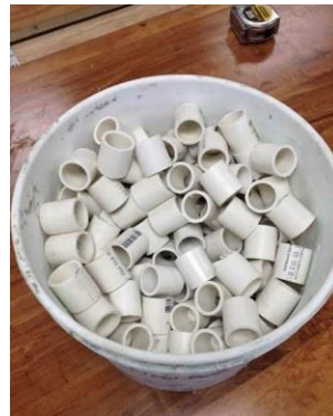
Figure 32: De-burred PVC pipe
