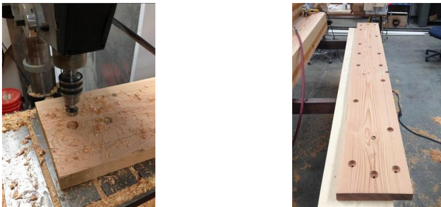
Figure 29: Drilling countersunk holes. Figure 30: Completed board though application process.
