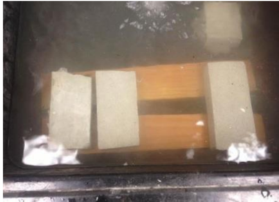
Figure 21: Test samples: no sealing, 1 sealing, 2 sealings, and 3 sealings submerged in water.
