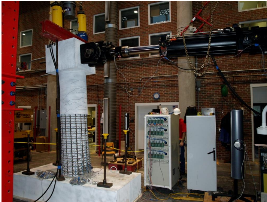
Figure 2.6 Specimen Under Lateral Deformation
