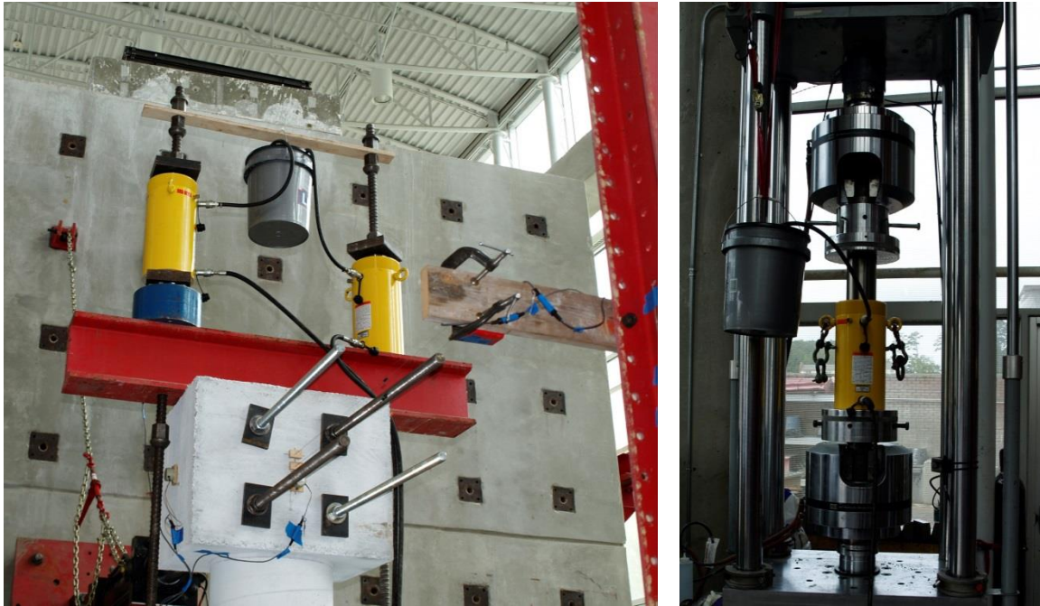
Figure 2.7 Self-Regulating Axial Load with 3 rd Jack in Force Controlled MTS Machine
