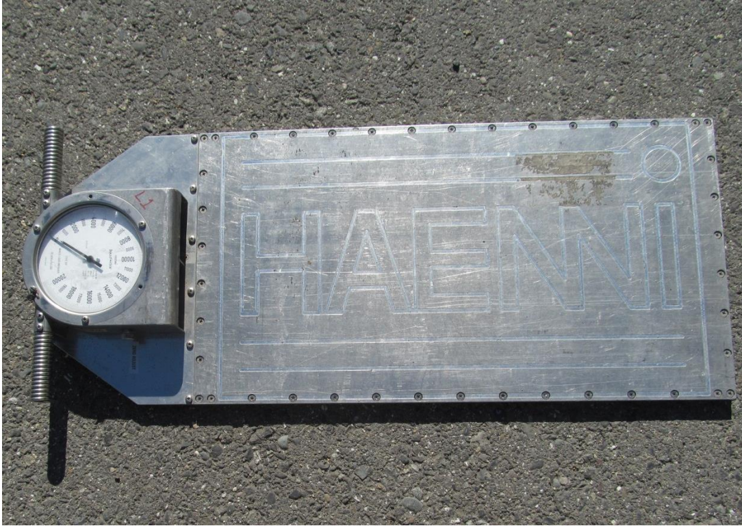
Figure I.7 Wheel load scales WL 101
