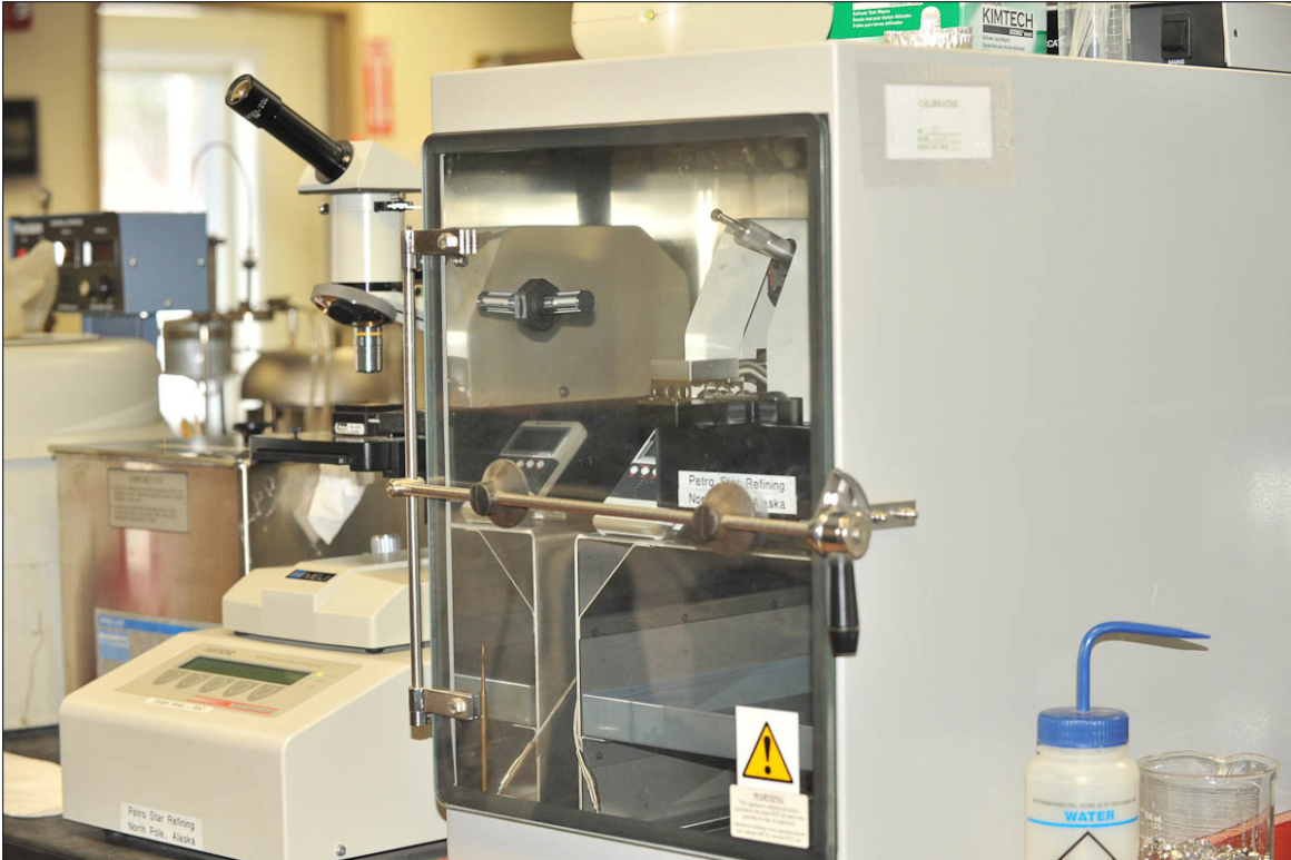
Figure 12. Scuff ball test rig, PetroStar laboratory. Enables PetroStar to measure the lubricity of its fuel and ensure that it meets ASTM D975 specifications. Photo by Frank Williams.
