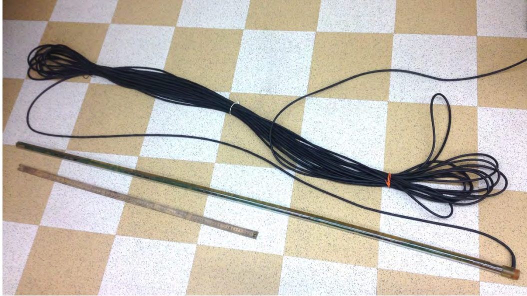
Figure 10. Thermistor array with its connection cable (the ruler placed alongside is 1 m long)
