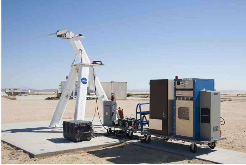
Figure 2: NASA Airvolt Test Stand. NASA’s propulsion device test stand to investigate the use of electric motors in aviation [14].
