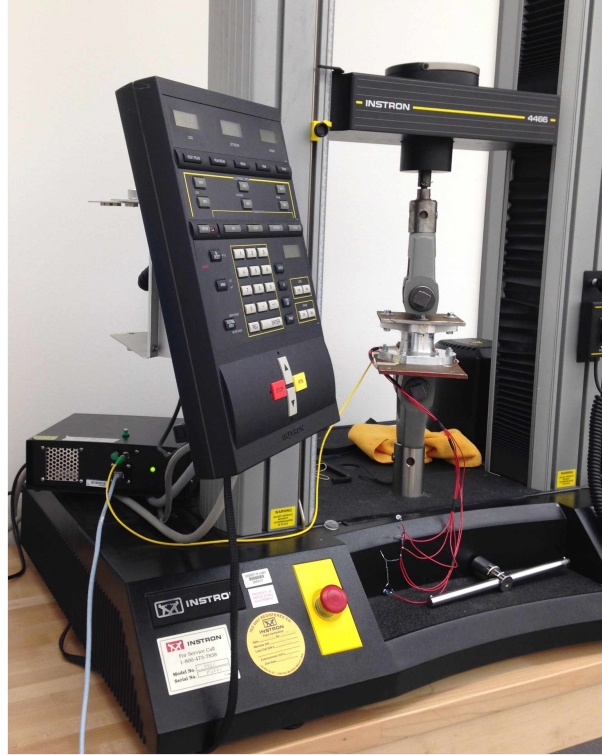
Figure 22: The load cell placed in the Instron Model 4400 to be loaded in tension for foil gauge system and fiber Bragg grating system calibration.
