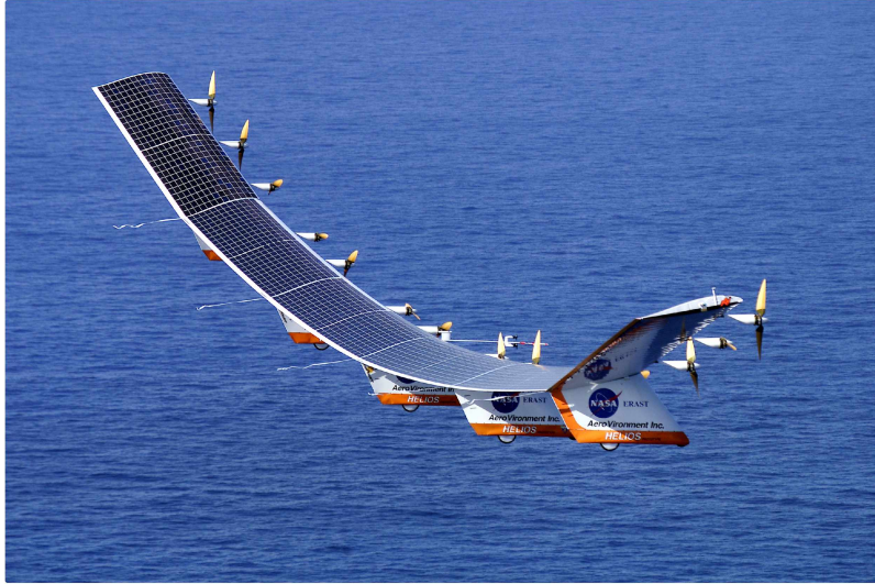
Figure 1: NASA Helios Prototype aircraft. Notice the multiple electric motors distributed along the wing [6].
