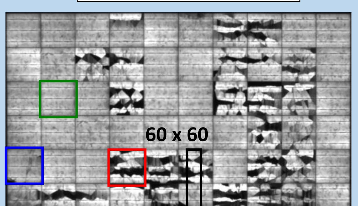
Maximum possible resolution for a (10 x 6 cells) panel allowed by a 640 x 512 camera
