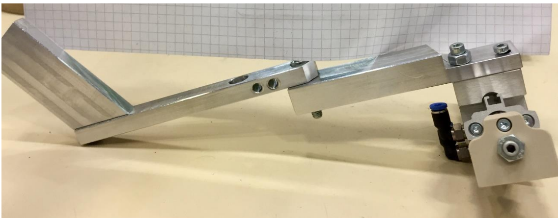
Fig. 4.4: Gripper holding structure use in the experiment
