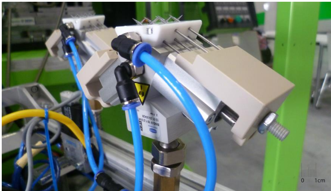
Fig. 3.4: Needle gripper in detail.
