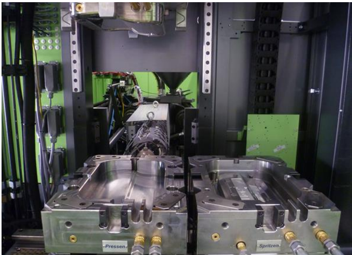
Fig. 3.6: Pressing unit opened with molds.
