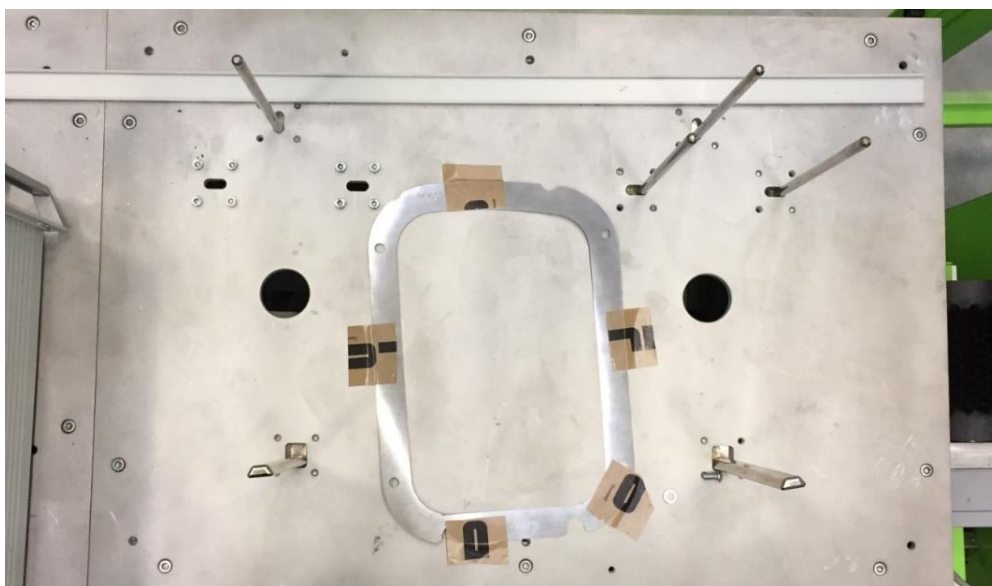
Fig. 3.8: Area where the machine will place the preform.
