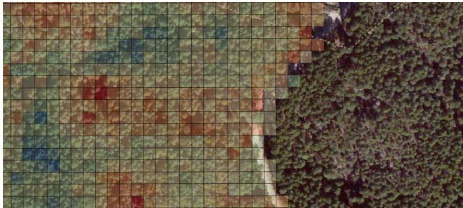
Figure 1. Example of LiDAR inventory cells with volume data and classification
