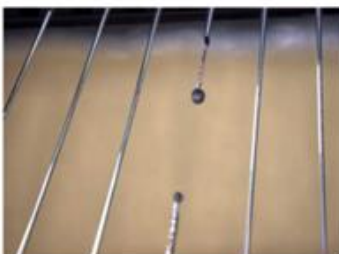
Melted bond wire
