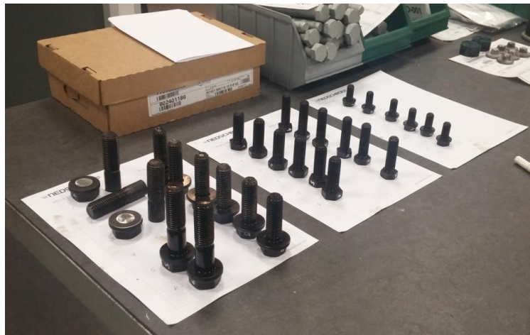
Figure 18. Bolts after hardening awaiting slicing and hardness testing
