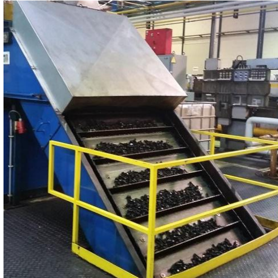
Figure 4. Products after quenching and on their way to the tempering furnace
