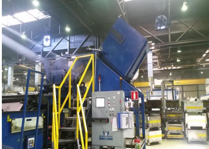
Figure 2. Loading of products onto Furnace #10 hardening belt via an automated hopper
