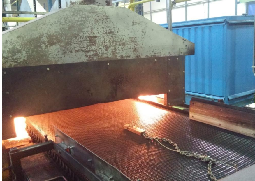
Figure 15. Steel block fitted with thermocouples, on the belt to enter the hardening furnace
