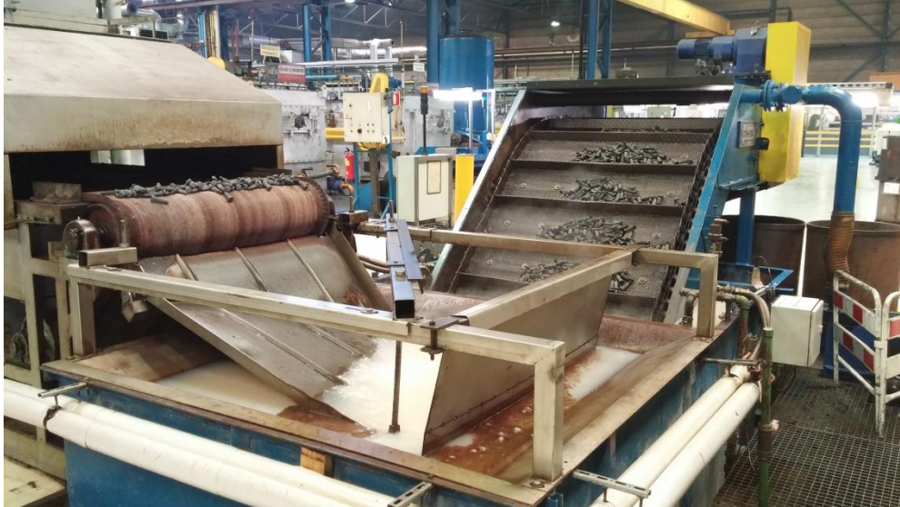
Figure 6. Products cooled in water emulsion and transferred to containers
