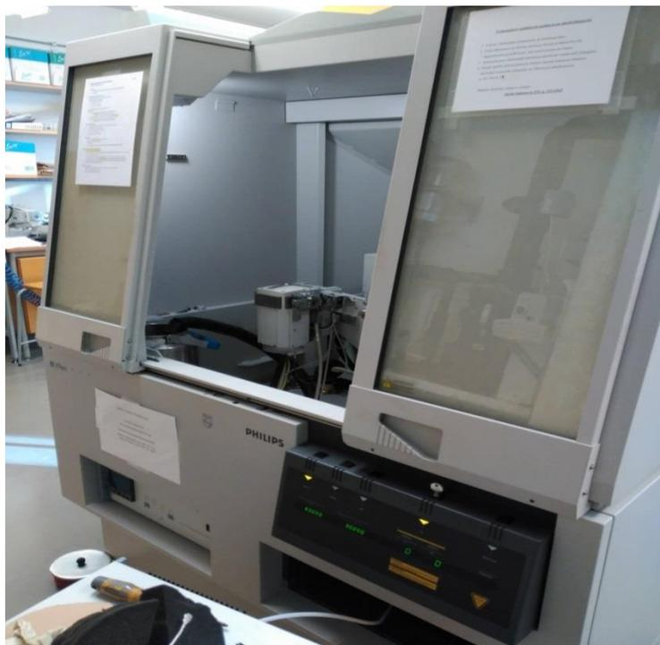
**Figure 05. Powder X-ray Diffraction (PXRD) equipment. University of Turku, Department of Physics and Astronomy.**
