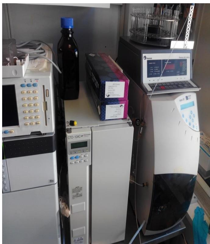
**Figure 03. Size-Exclusion Chromatography (SEC) equipment. Åbo Akademi University (ÅA). Laboratory of Wood and Paper Chemistry.**
