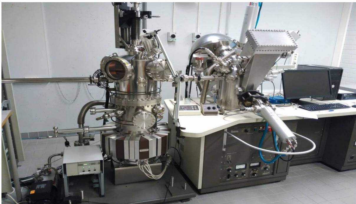
**Figure 07. X-ray Photoelectron Spectroscopy (XPS) equipment. University of Turku. Department of Physics and Astronomy.**
