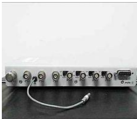
Figura 25 HP Agilent 35670A/U UK4 Option Microphone Adapter
