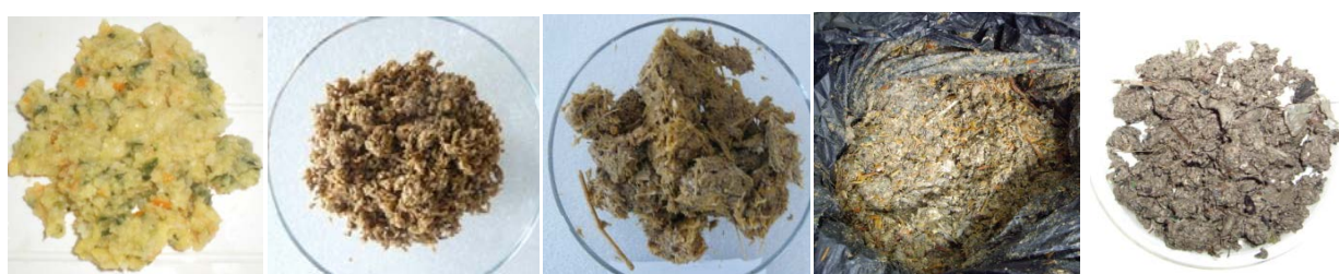
Substrates (from left to right): Organic fraction municipal solid waste, spent grain, cow manure, grease waste and pre-selected municipal solid waste.
